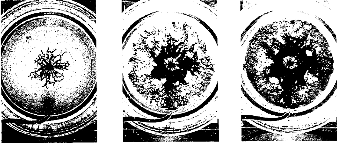
Fig. 6a- Imbibition caused by high P_c (low N_{ca} ) followed by end effects (low K , high IFT and low Q ) c .
