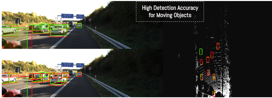
FIGURE 6.8: A scenario from KITTI [6] shows our network’s high detection accuracy for moving cars. GT: green, PRED: red.
