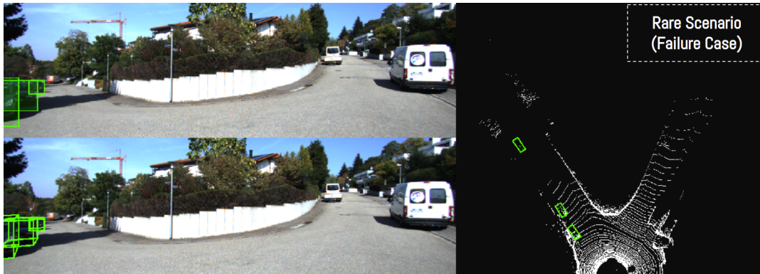
FIGURE 6.6: A rare scenario from KITTI [6] that is tricky to our fusion network and yields a failure case. GT: green, PRED: red.
