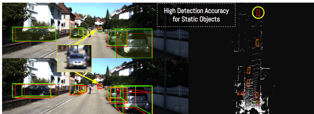
FIGURE 6.9: A scenario from KITTI [6] that shows our network’s high detection accuracy for non-moving cars. GT: green, PRED: red.
