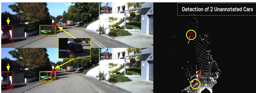
FIGURE 6.11: Another scenario from KITTI [6] where 2 unannotated cars were correctly detected by our fusion network. GT: green, PRED: red.
