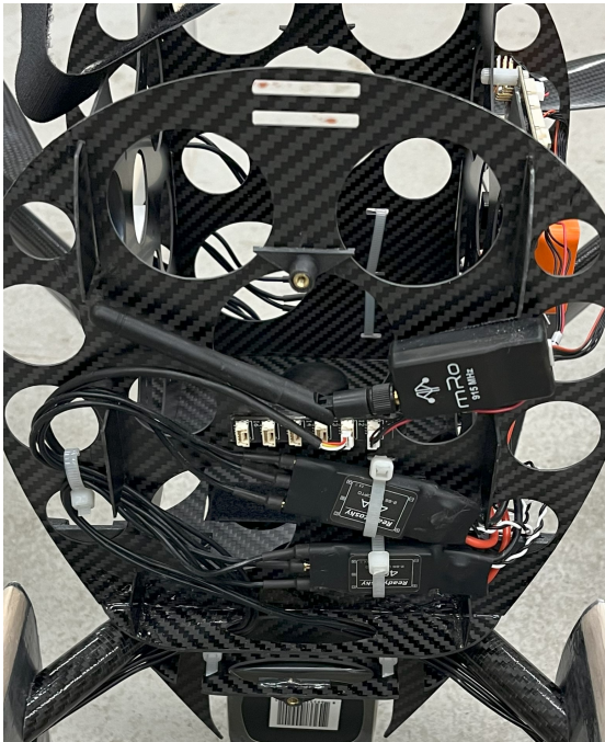
(c) Side of payload bay showing two ESCs and radio mounting.
