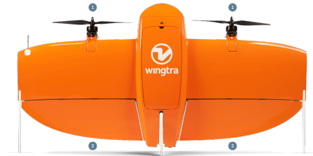
(b) The WingtraOne commercial tailsitter for surveying with two rotors and two control surfaces [139].
