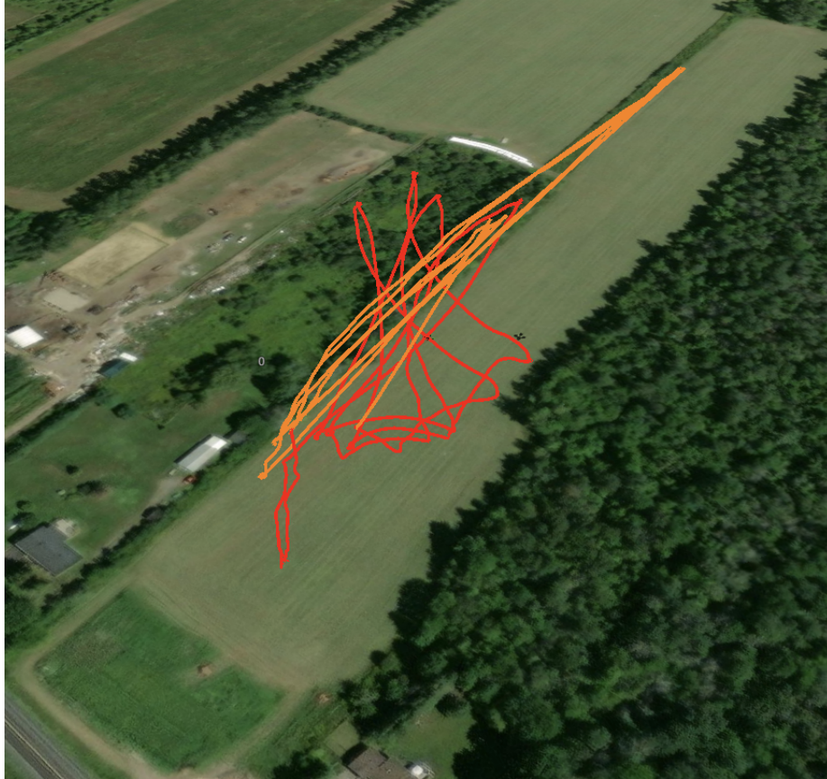
Figure 5.2: Flight path and location for flight 11 testing. The red lines represent passes made in loiter mode with manual control, and the orange lines are GPS waypoint passes in guided mode.
