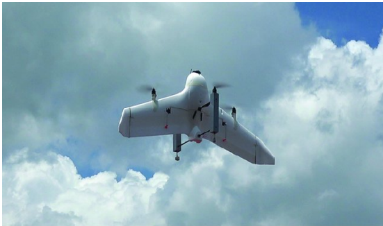
(c) Modified SkywalkerX-5 tailsitter with four rotors and two control surfaces [64].
