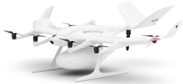
(b) The Wingcopter 198 tiltrotor delivery drone with 8 rotors, 4 actuators to tilt the rotors, and 4 control surfaces [137].
