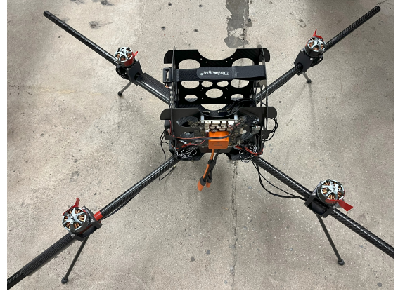
(b) Zoomed out view including motors and diagonal carbon fibre tubes.
