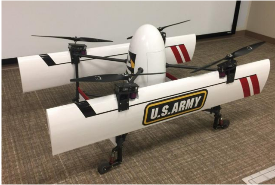
(a) U.S. Army prototype tailsitter with wings mounted underneath a rigid quadrotor frame [17].
