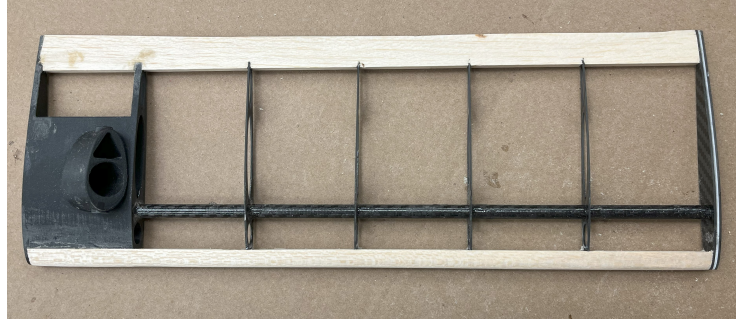
Figure 2.23: Short wing segment showing carbon fibre ribs and spar, balsa leading and trailing edges, and 3D printed mount.
