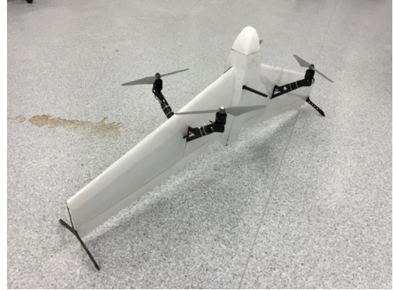
(b) A single-winged tailsitter with four rotors and two control surfaces [136].
