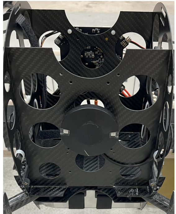
(d) Top of payload bay showing the GPS position and mounting.
