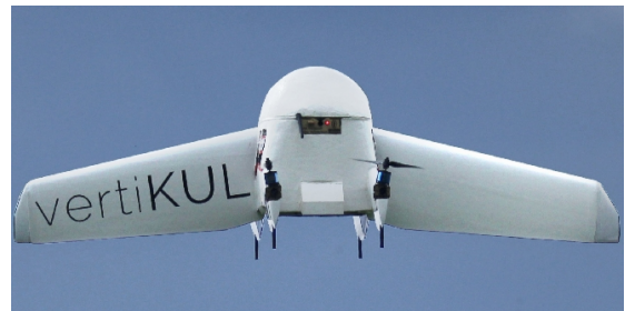
(d) VertiKUL tailsitter for payload delivery with four rotors and a fixed wing [58].
