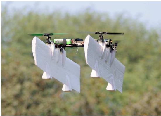
(c) A biplane tailsitter with four rotors and no control surfaces [33].
