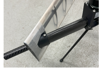
(c) Wing mounting on carbon fibre diagonal tube.
