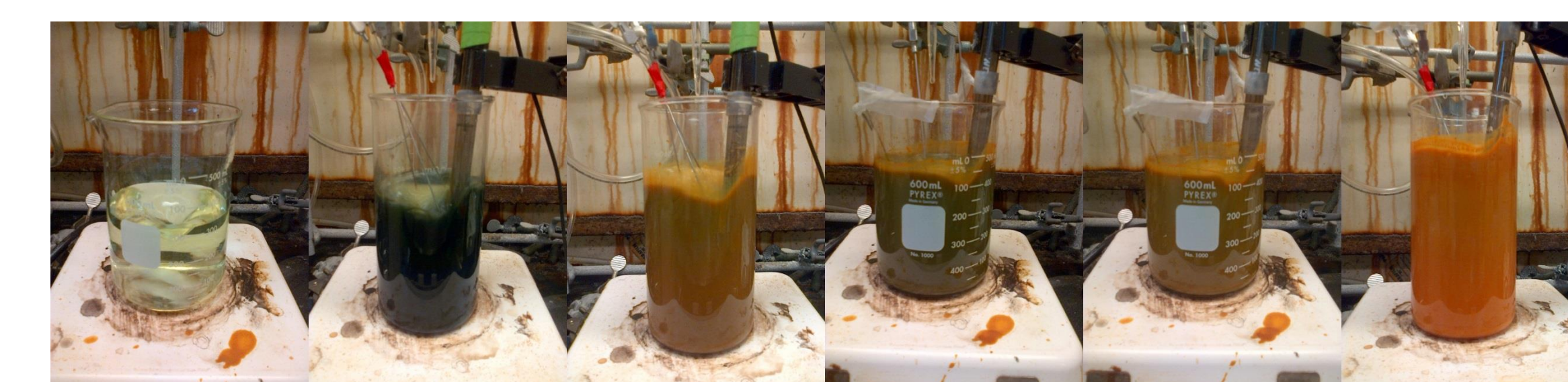
Figure 3. Lepidocrocite without alginate synthesis. (Left to right) 11.93g of FeCl 2 was added to 400mL of Millipore water (pH ~3). The ferric chloride solution was brought up to ~6.7 pH with 1 M NaOH. Solution was allowed to oxidize with a constant airflow: 30 mins of airflow; 1 hour; 1 hour and 15 mins; and ~2 hours of airflow with a grand total of ~120 mL of 1 M NaOH added.
