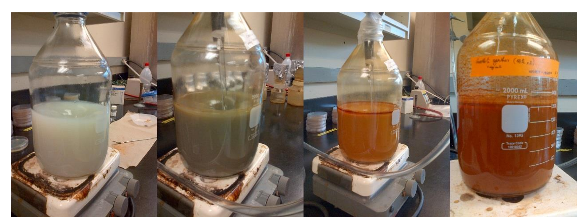
Figure 2. Goethite without alginate synthesis. (Left to right). FeCl 2 with bicarbonate solution with no airflow added, 30 mins of airflow, 18hrs of airflow, 3 days and 18 hrs of airflow.
