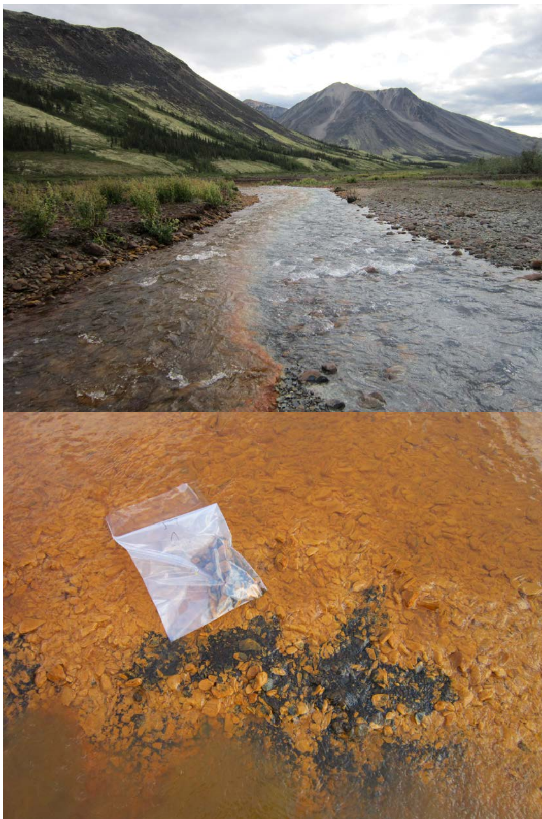
Figure 13. Ferrhydrite precipitation downstream of the confluence of low pH waters sampled at T3 and neutral waters sampled at SM4.
