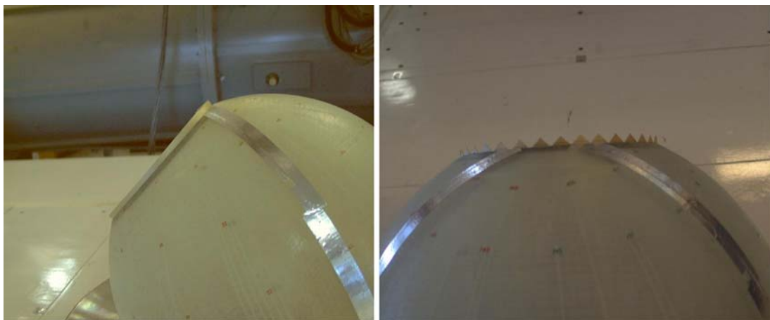
Figure 4.54 1 cm-high opening lip (left) and 1 cm-high-serrated lip (right).
