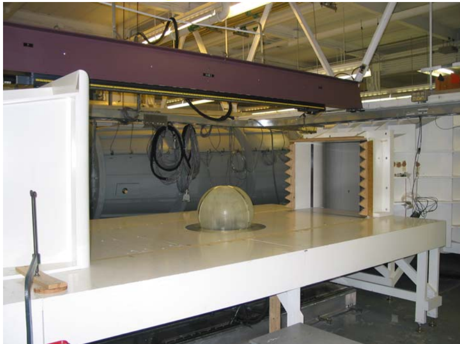
Figure 4.1 The telescope ensemble and its position inside the pilot wind tunnel (after Cooper et al 2004).
