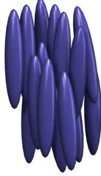
Figure 2.10: Long, rod-shaped liquid crystal molecules aligning in nematic phase.
