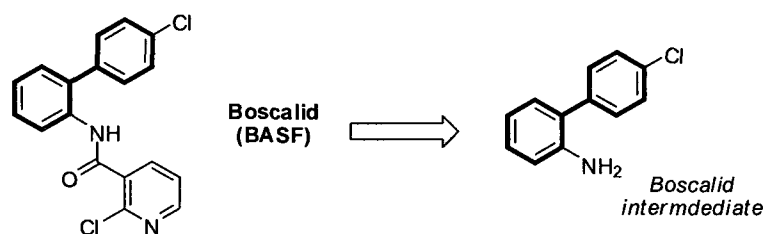
Scheme 3-8: Retrosynthesis of Boscalid demonstrating the key intermediate
