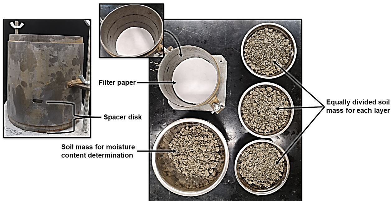
Figure 4-1 Illustration of compaction procedure for specimens tested in saturated and w_{opt} condition
