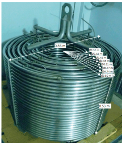
Figure 1.1. 73 L plug flow reactor used at Eli Lilly for the continuous flow hydrogenation of enone 1.5 . Image reproduced from ref 14a with permission from ACS publications. 15
