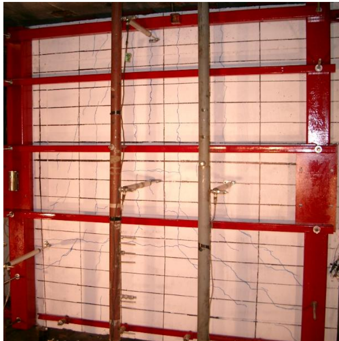
Figure 6.16: Condition of Wall 1 after test 4
