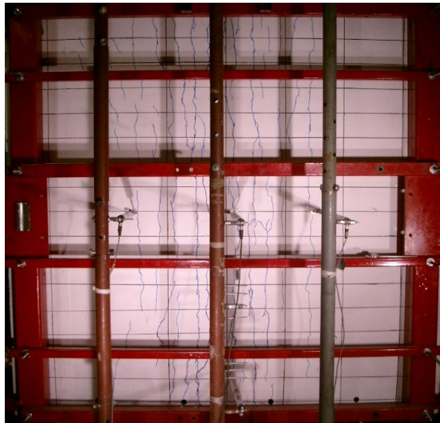
Figure 6.48: Condition of Wall 2 after test 6
