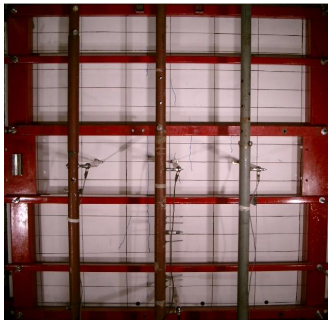
Figure 6.36: Condition of Wall 2 after test 3
