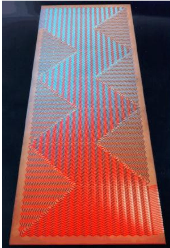
Figure 2-12 [9] Typical Printed Circuit Heat-exchanger Plate (Heatric Ltd)
