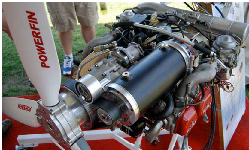
Figure 2.3.: Parallel hybrid propulsion system for a fixed-wing aircraft [24, 25]
