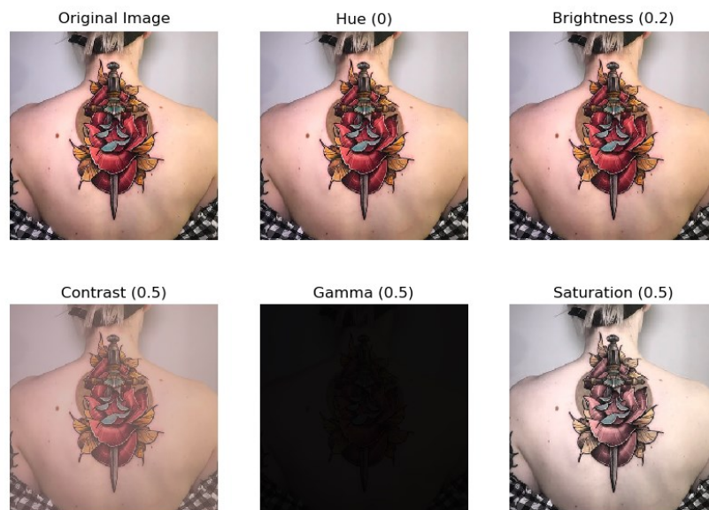
Figure 11 - Segmentation Data Augmentation (Lower bound). This image shows the result of the 5 alteration types using the lower bound values of the random range used when making the augmentation during training. Image used in this figure [204] is in the public domain.
