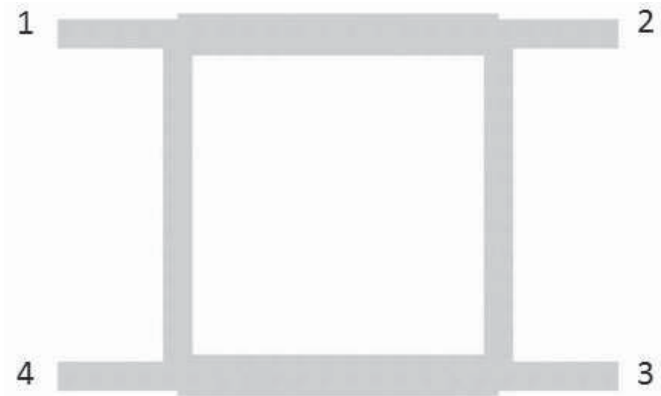
Figure 5.10: Geometry of 90° hybrid coupler.
