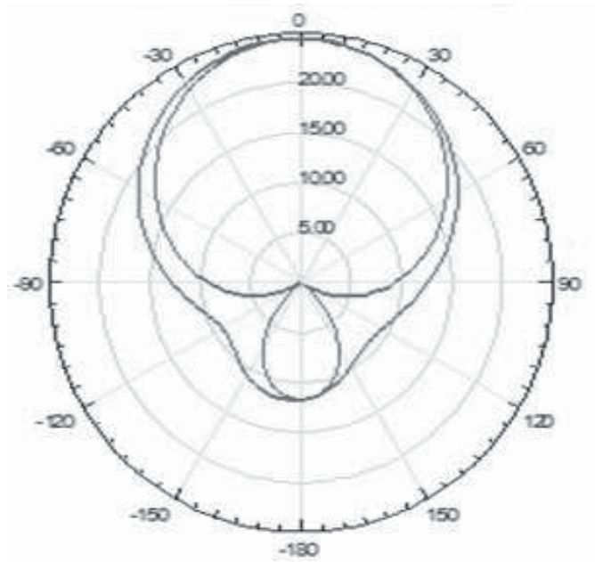
Figure 4.5: Radiation pattern at 2.45 GHz (single-band).
