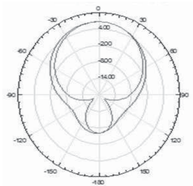
Figure 4.9: Gain at 2.45 GHz (dual-band).
