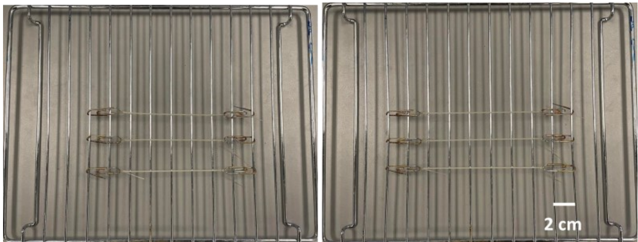
Figure 13: Pre-stretch introduced in TCP samples: (left) Before annealing; (right) After one hour of annealing
