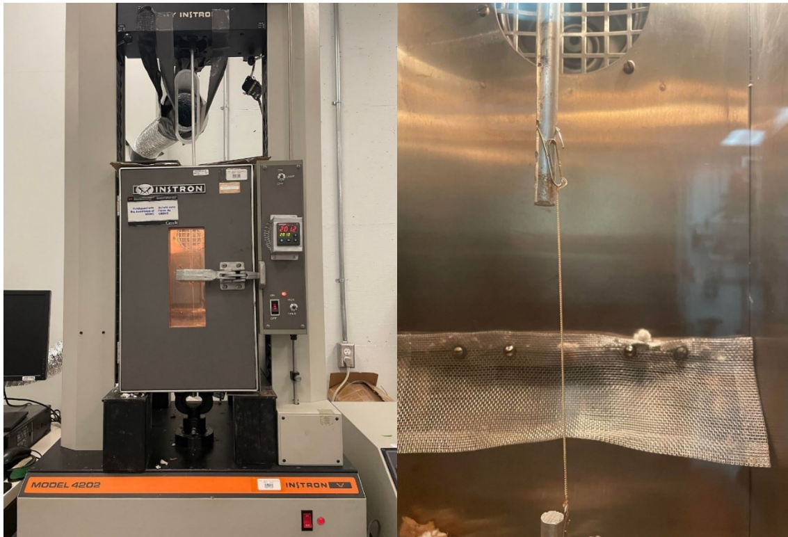
Figure 10a) Experimental setup for isometric and eccentric contractions; b) Inside view of environmental chamber with TCP sample ends fixed
