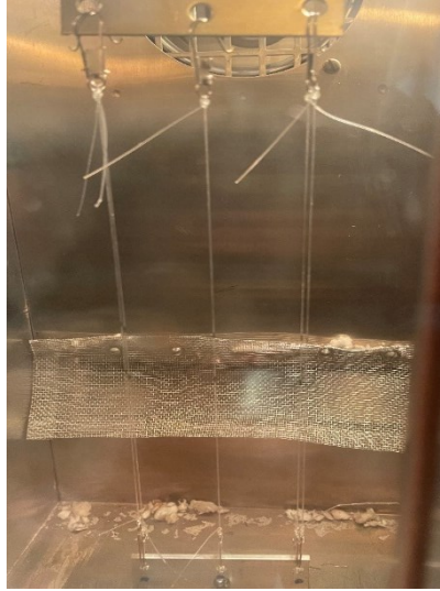
Figure 59: Inside view of Instron environmental chamber with precursor fibres being stretched to 5% and annealed
