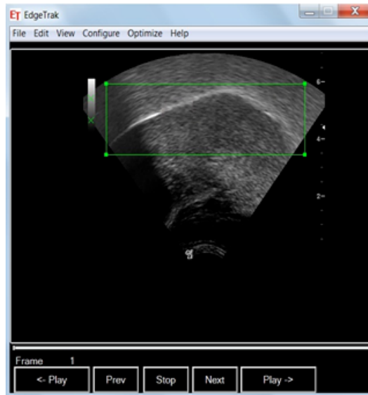
Figure 29: Adjustment of the target area (green region) and setting the image gradients.
