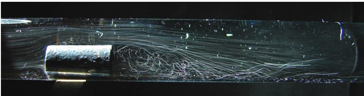
Figure 3 - 17 Flow visualization by hydrogen bubbles around 30B obstacle, Re=3000 .
