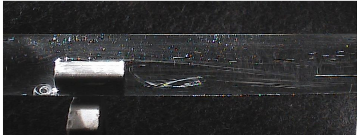
Figure 3 - 13 Flow visualization by hydrogen bubbles around 30B obstacle, Re=700 .
