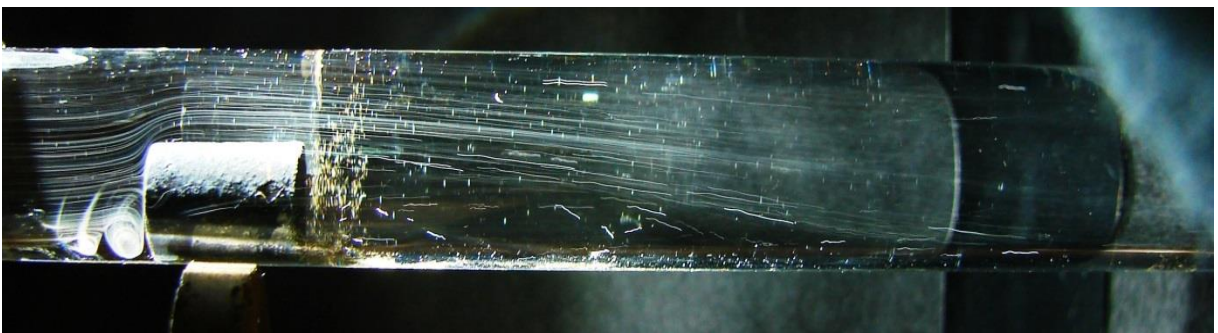
Figure 3 - 14 Flow visualization by hydrogen bubbles around 30B obstacle, Re=1400 .
