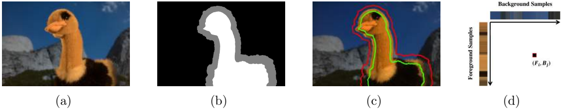
Figure 3.3: (a)The original image[3], (b) one possible trimap, (c) FG(green) and BG(red) dictionaries and (d) the pair-space with a square depicting a particular pair in it.
