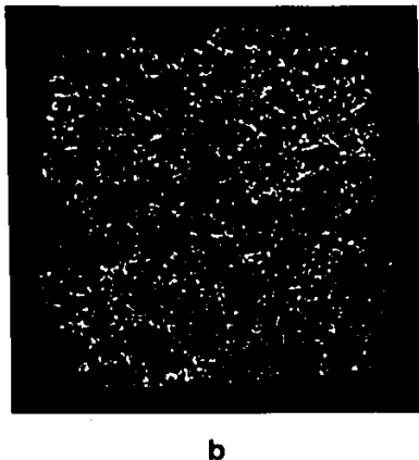
Figure 8.26: (a) portion of the thin section of amphibolite which was studied. The study area is indicated by arrows; the trace of the foliation plane is horizontal. The letters h, b, and p, indicate hornblende, biotite and plagioclase crystals, respectively; (b) the boundary tracing of all grains in the study area.
