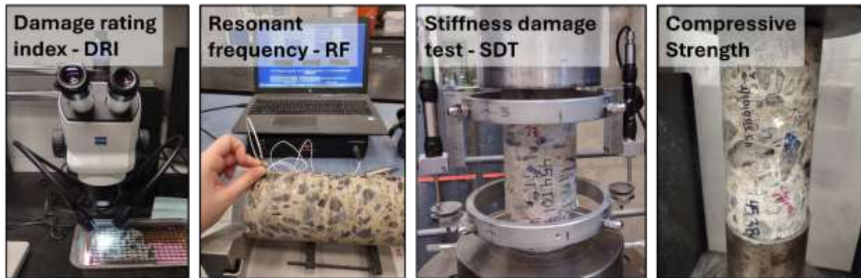
Figure 3-9 Images depicting the damage rating index (DRI), resonant frequency (RF), stiffness damage test (SDT) and compressive strength tests used in analysis of core specimens
