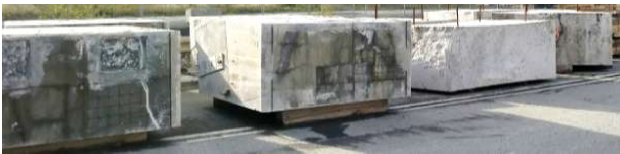
Figure 3-3 Image depicting segments of the pier cap (left two segments) and pier shaft (right two segments) at the Montreal storage site
