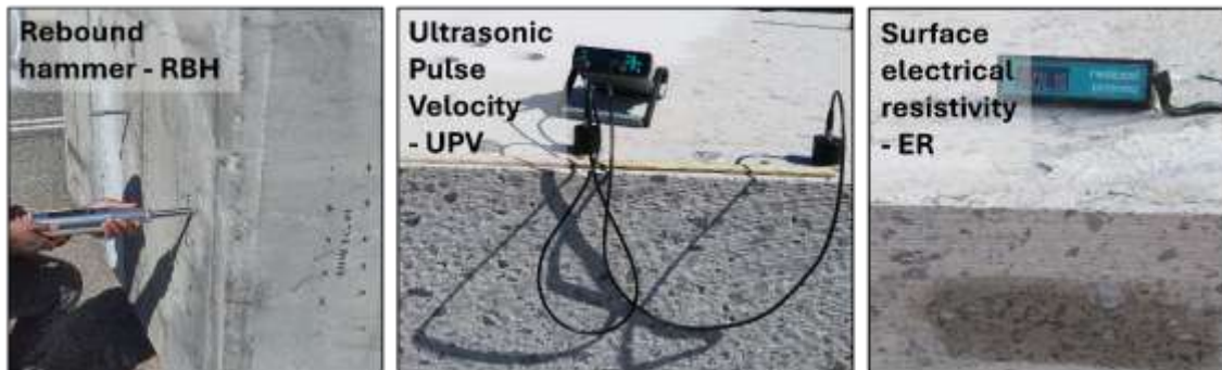
Figure 3-5 Images depicting the rebound hammer (RBH), ultrasonic pulse velocity (UPV) and surface electrical resistivity non-destructive testing techniques
