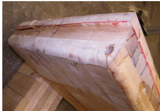
Figure 4.56: CLT3-4 Shear Failure
