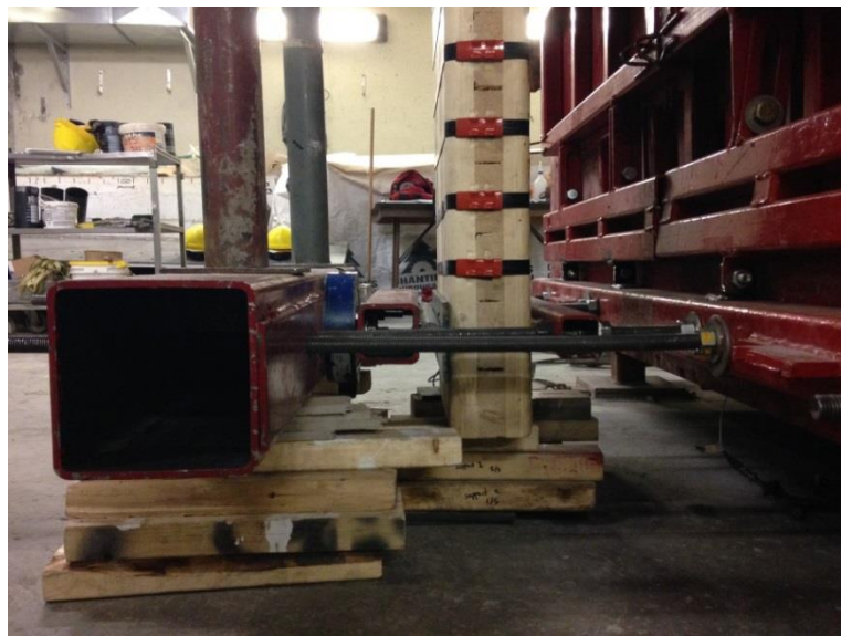
Figure 3.27: Simply Supported End Condition Detail
