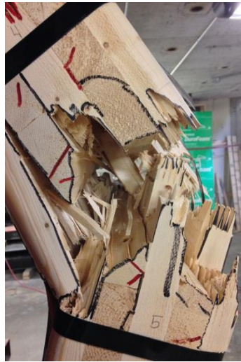
(a) Finger Joint on Laminate 1
