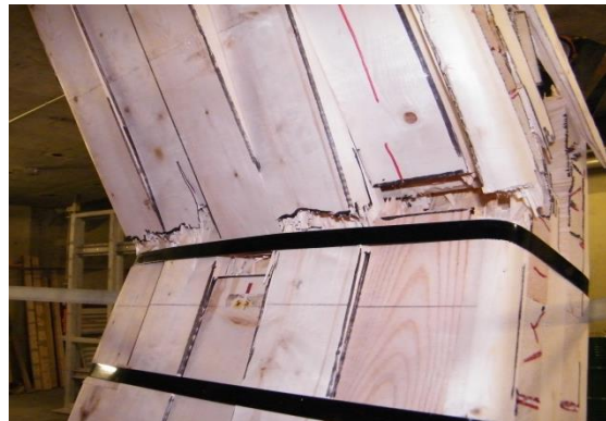
Figure 4.36: CLT5-5 Compression Failure
