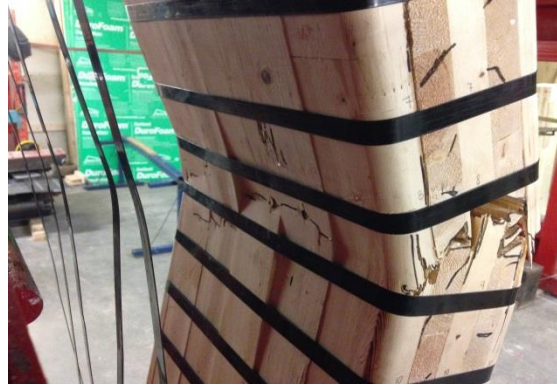
Figure 4.22: CLT5-1.2 Compression Failure
