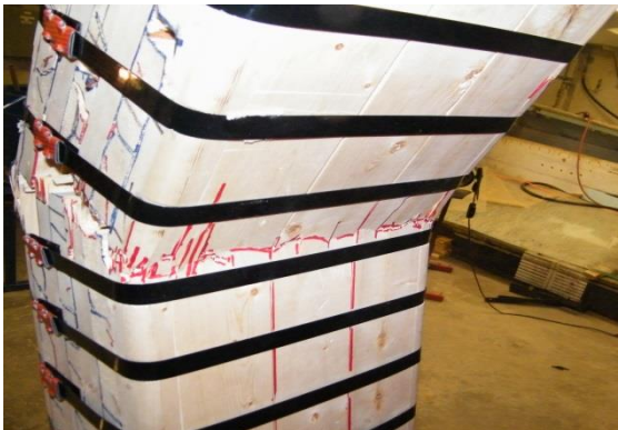
(a) Compression Failure
