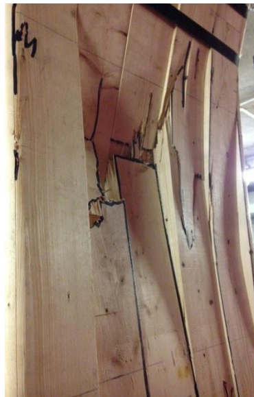
Figure 4.17: CLT3-2 Compression Failure
