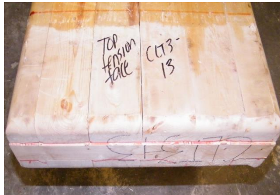
Figure 4.53: CLT3-3 Shear Failure
