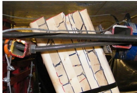
(b) Shear Failure
