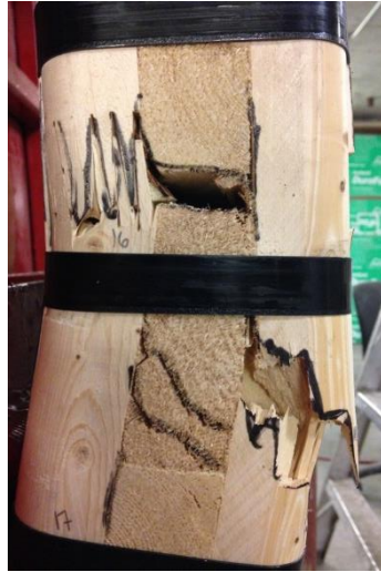
(a) Finger Joint on Laminate 1
