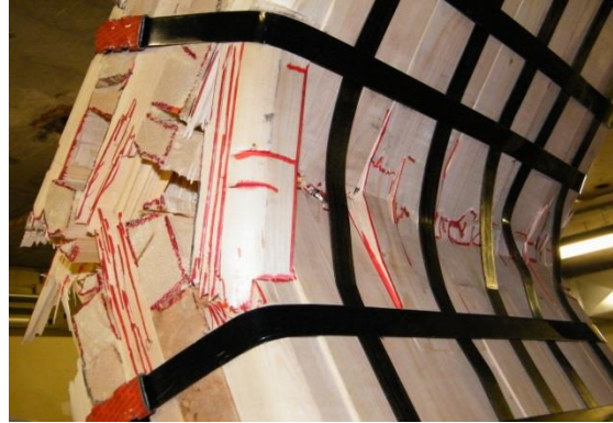
Figure 4.27: CLT5-2.2 Compression Failure
