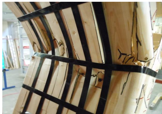
Figure 4.33: CLT5-4 Compression Failure
