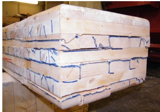
Figure 4.70: CLT7-D2 Shear Failure
