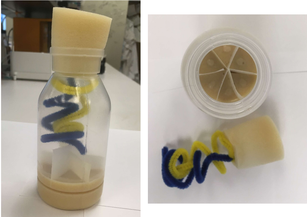
Fig. S2.1. Side and top view of the complex mating environment for our population of Drosophila melanogaster . The environment is made of a polypropylene bottle filled with 75 ml of food. The surface of the food is divided into six approximately equal sectors delimited by opaque plastic barriers inserted into the food. Equal amount of liquid yeast was dropped in each food patch. In addition, two coiled pipe cleaners protrude from the bottom of the foam plug into the interior space of the bottle.
