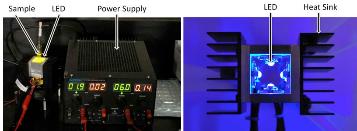
Figure 2.4: Experimental setup for controlling the shape of AgNP formed from AgNP seeds, setup on the left and zoomed in LED/heat sinks on the right.
