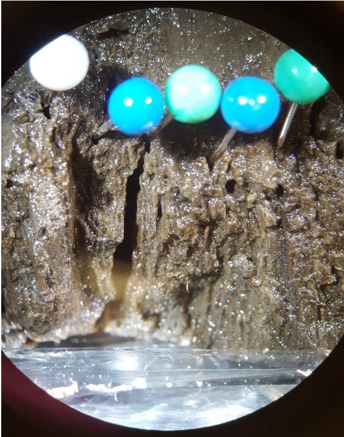
Figure 3.3 Magnified view of the annual laminations (varves) from Lac Noir sediment core using a Leica Wild M3C stereo microscope. Coloured pins represent 10-yr intervals. Picture taken by Dr. K. Neil (2017)
