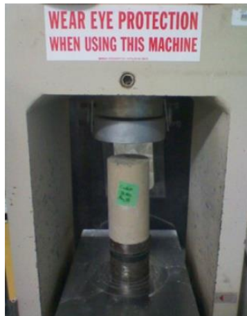
(a) Cylinder testing machine
