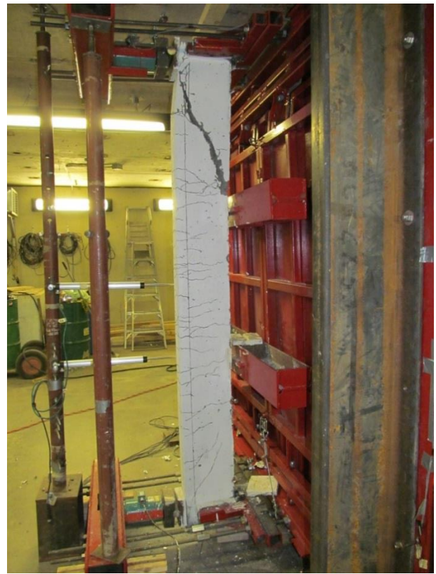
(c) SCC 1.5% 5D shear failure at Blast 3
