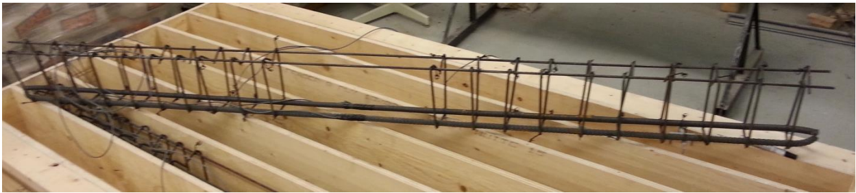
Figure 3.6 typical cage with stirrups
