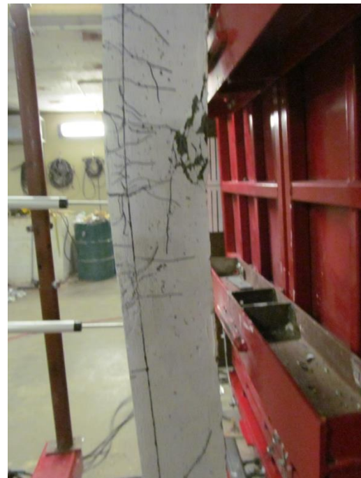
(b) Mid-Span Results of Blast 4
