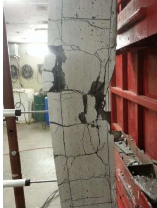
(b) Mid-Span Result of Blast 4
