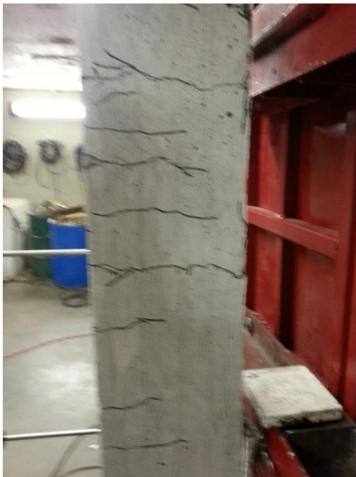
(a) Mid-Span Results of Blast 3
