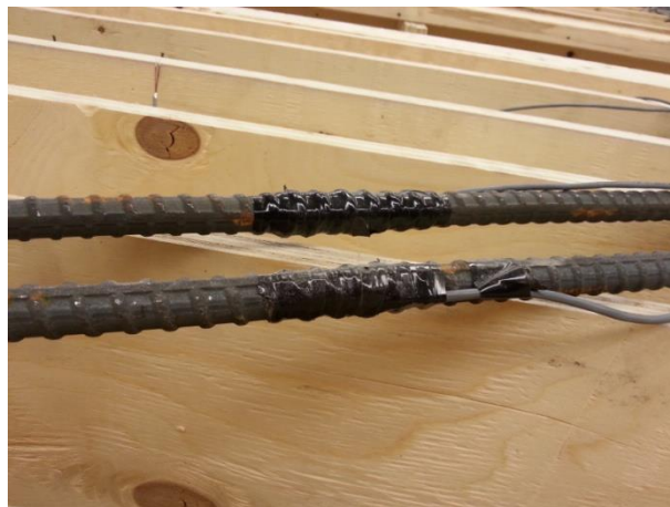
Figure 3.7 Typical bars sowing strain gauge instrumentation
