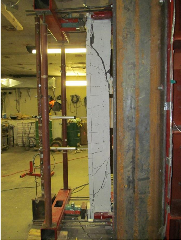
(a) SCC 0% mm shear failure at Blast 2
