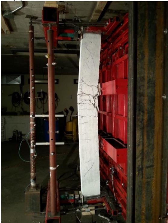
(e) SCC 1% ZP flexural failure at Blast 4
