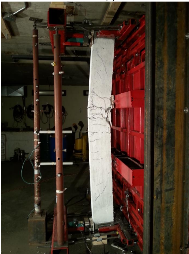
(b) SCC 1% ZP flexural failure at Blast 4
