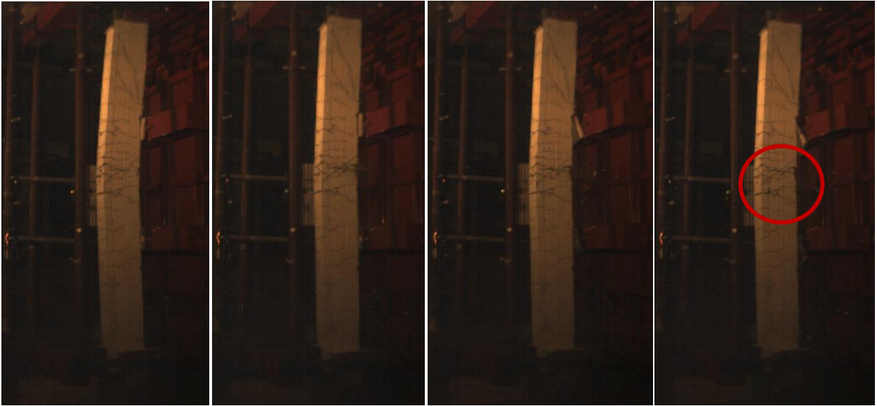
Figure 5.40: SCC 1% - Secondary Fragmentation
