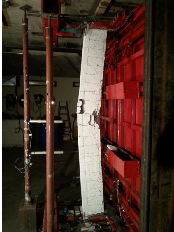
(a) SCC 0% 100mm flexural failure at Blast 4
