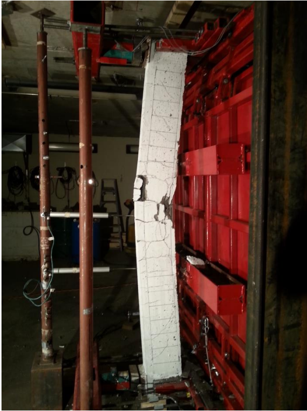
(a) SCC 0% 100mm flexural failure at Blast 4
