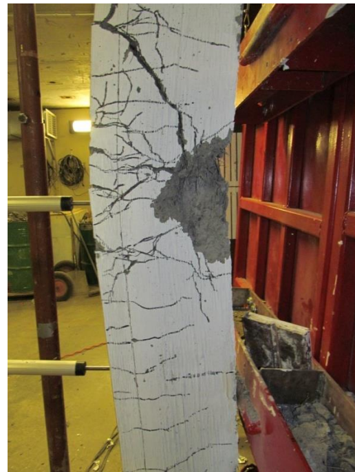
(b) Mid-Span Results of Blast 5
