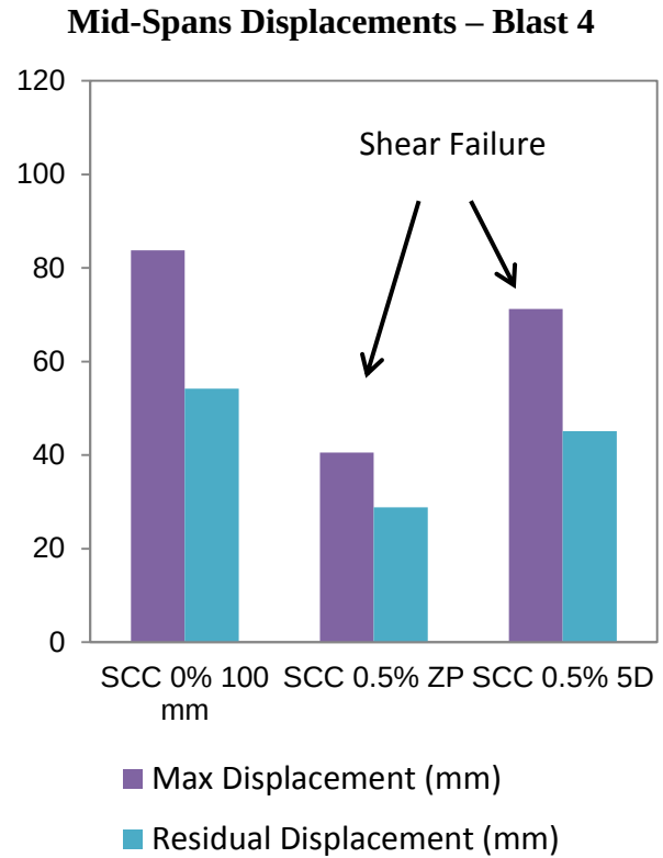
Figure 5.26: Maximum and residual displacements; effect of fiber type (0.5% fiber ratio)
