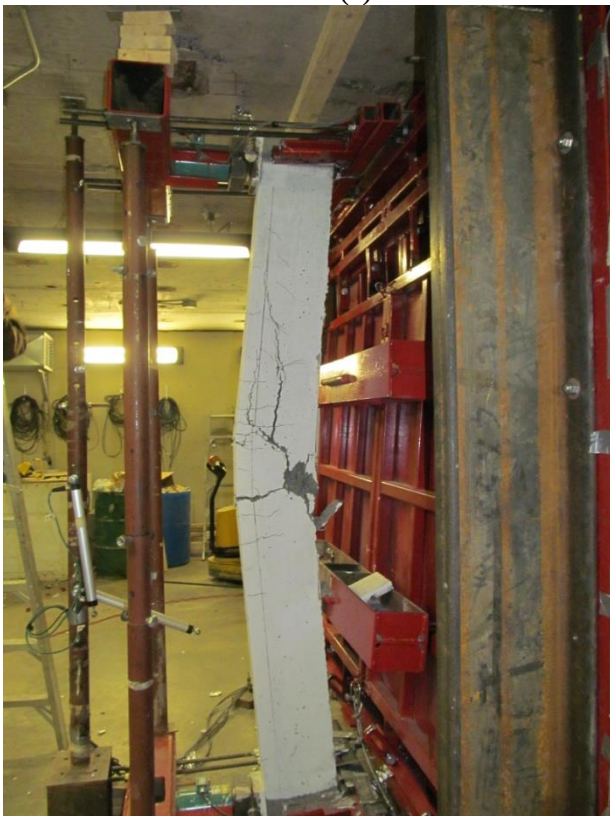
(b) SCC 1.5% ZP flexural failure at Blast 4
