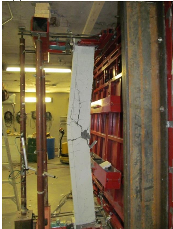
(f) SCC 1.5% ZP flexural failure at Blast 4
