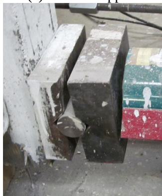
(b) Bearing plate and roller
