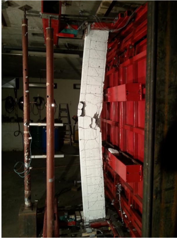
(a) SCC 0% 100mm flexural failure at Blast 4
