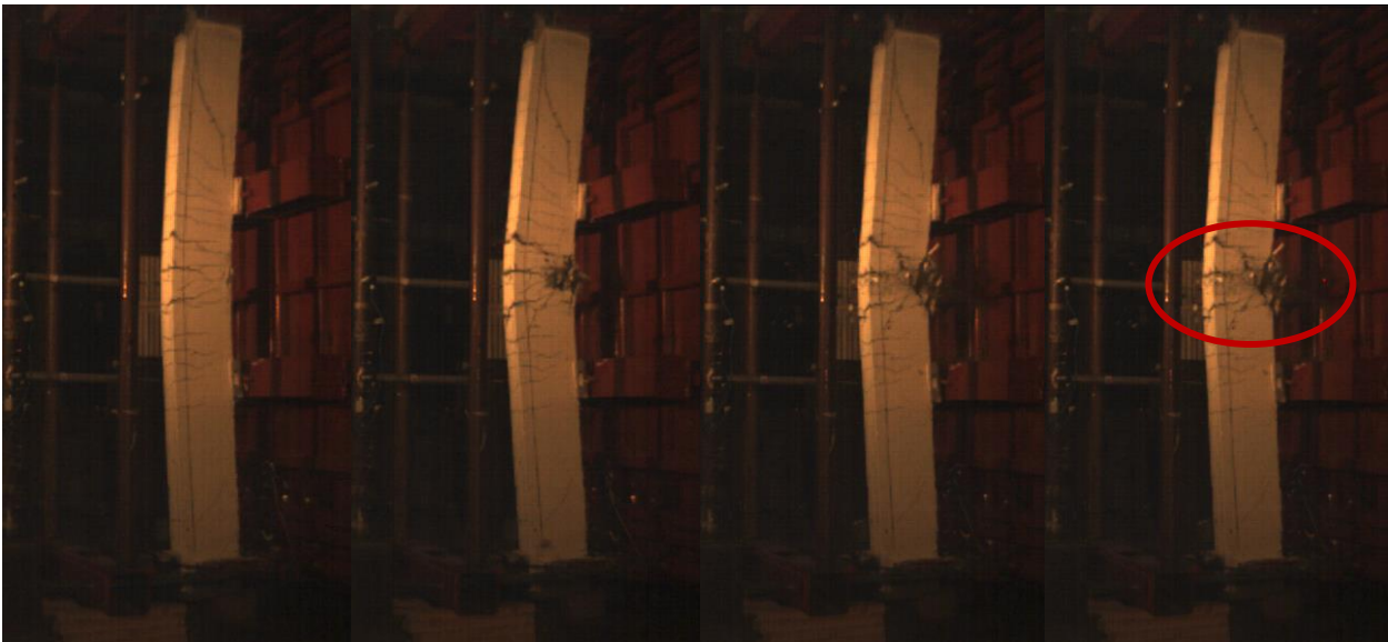
Figure 5.41: SCC 0.75% BP – Secondary Fragmentation
