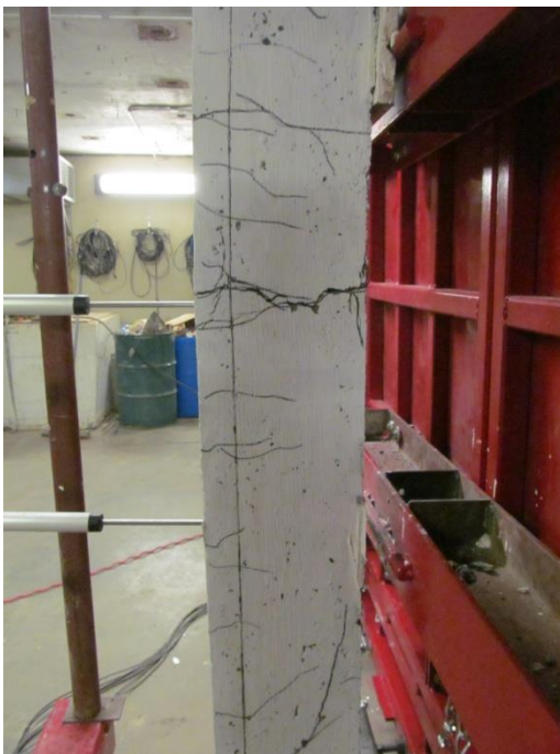
(a) Mid-Span Result of Blast 3
