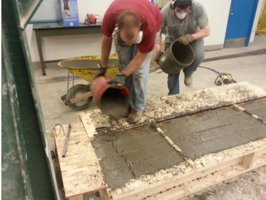
Figure 3.9 Placing of the beams
