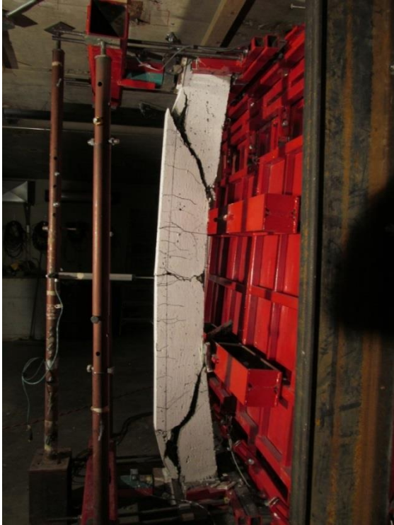
(c) SCC 0.5% ZP shear failure at Blast 4
