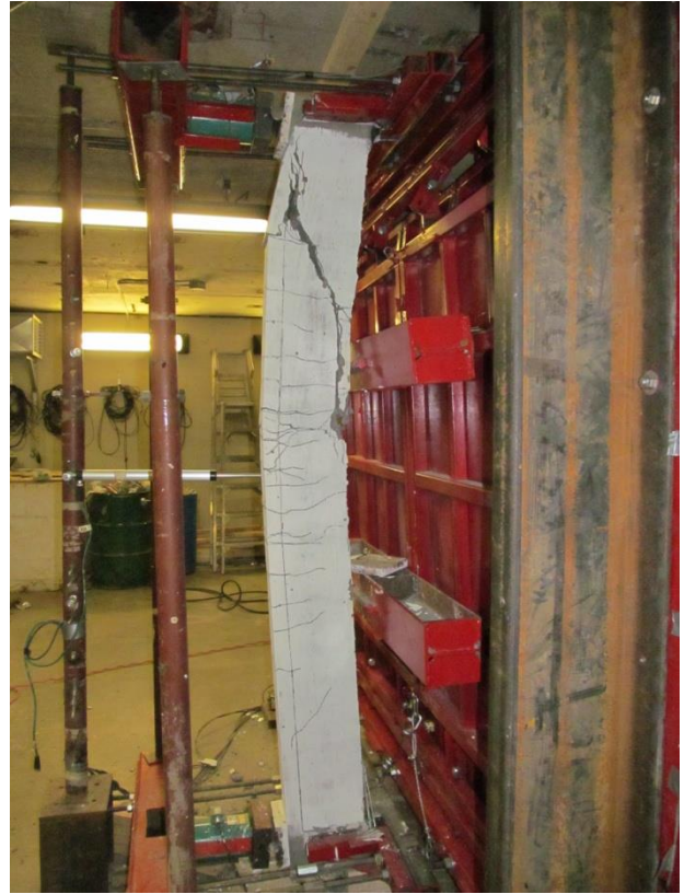
(b) SCC 0.5% 5D shear failure at Blast 4
