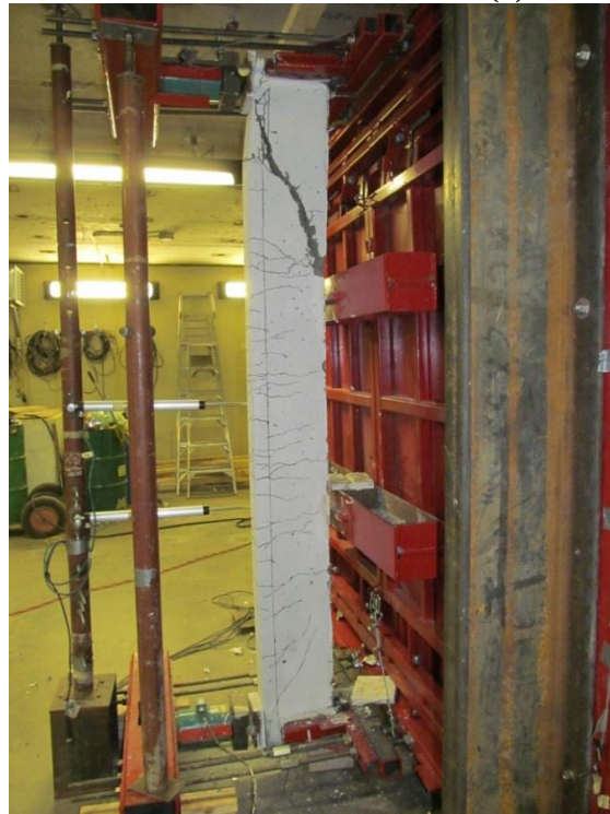
(e) SCC 1.5% 5D shear failure at Blast 3
