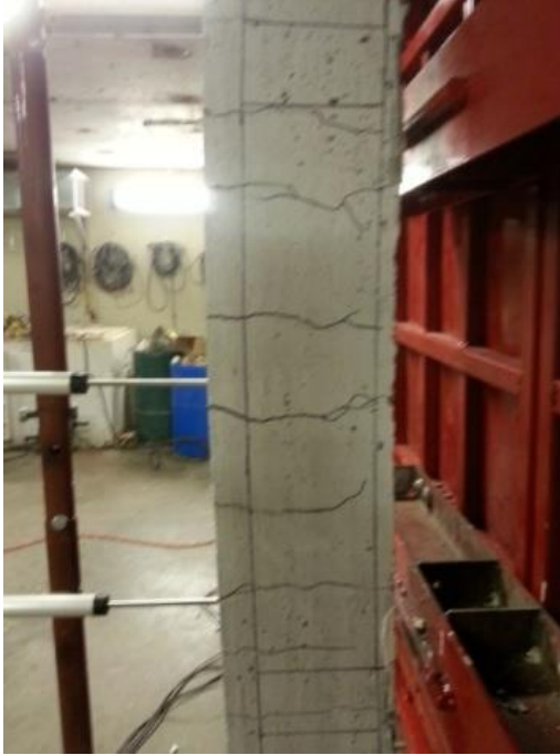
(a) Mid-Span Result of Blast 3
