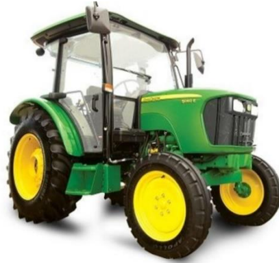
Figure 2.9. Two-wheel drive tractor (Copyright 2025 by Deere and Company).
