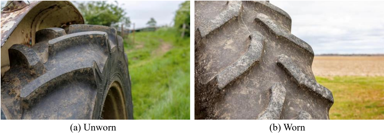
Figure 1.2. Closeup of the lugs on an unworn versus a worn tractor tire (Copyright 2025 by Alamy Limited).
