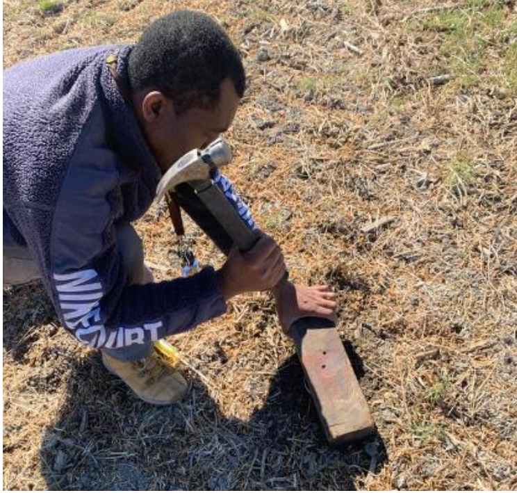
Figure 3.10. Cylindrical core being pounded into the soil for sample collection.
