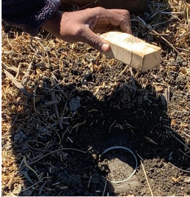
Figure 3.9. Collecting a soil sample using the cylindrical core.
