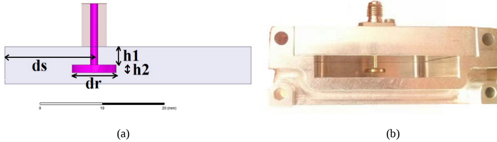
Fig. 4-13: Structure of the waveguide to coaxial adapter, (a) simulation drawing (side view) and (b) manufactured prototype (front view)
