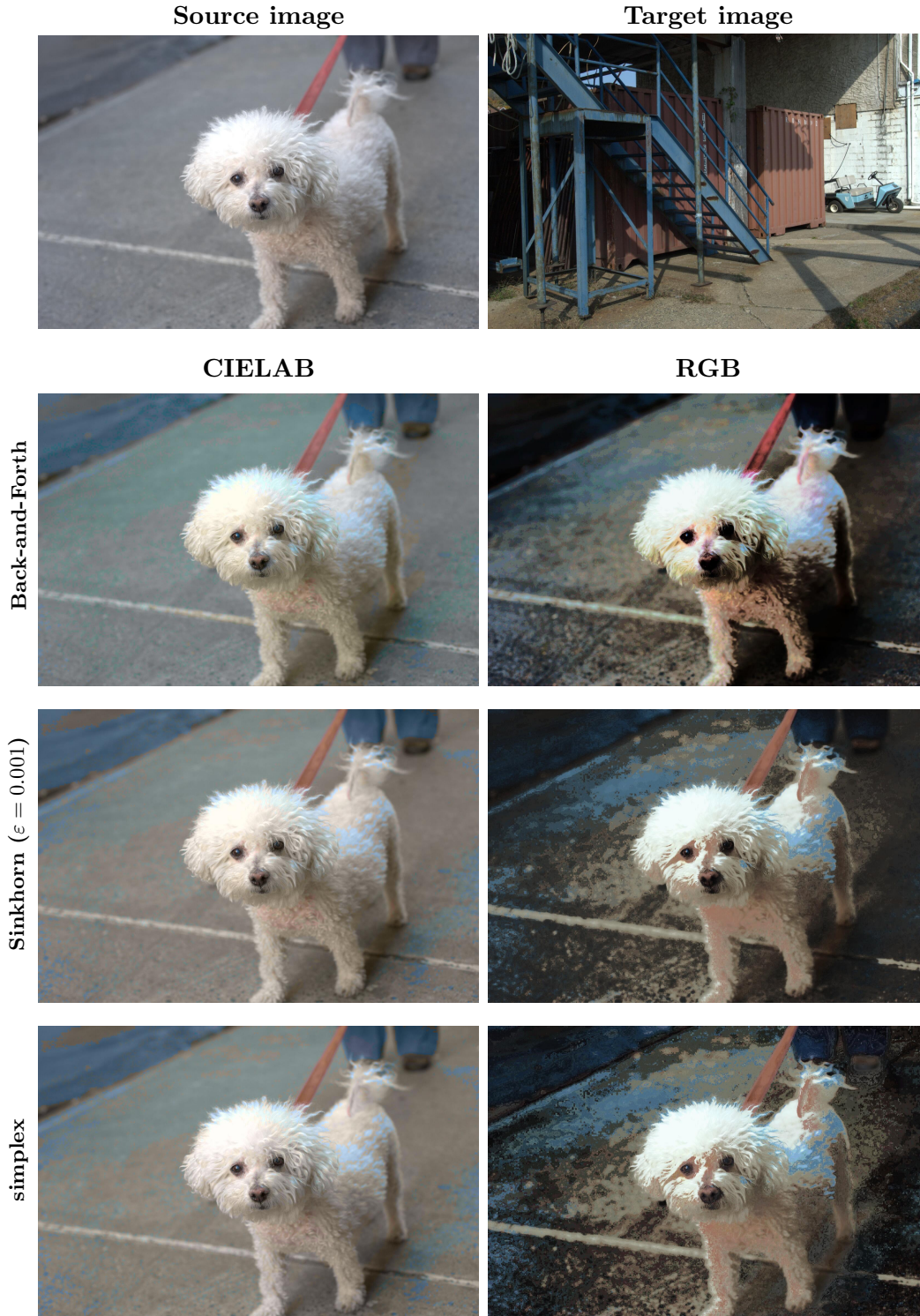
FIGURE 27. Comparison of constant cell-like artifacts across solvers. The first row shows the source and target images. The remaining rows compare recolouring results produced by the Back-and-Forth, Sinkhorn, and simplex solvers in CIELAB and RGB colour spaces. Visually, the simplex solver, which computes the exact histogram matching result on the discrete support, produces the strongest piecewise-constant cell-like artifacts. These artifacts are less visible for Sinkhorn and are reduced most clearly for the Back-and-Forth method, whose outputs appear smoother overall.
