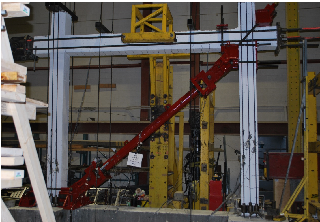
Figure 7.79: Cracking pattern at 1.5% lateral drift for Frame RF
