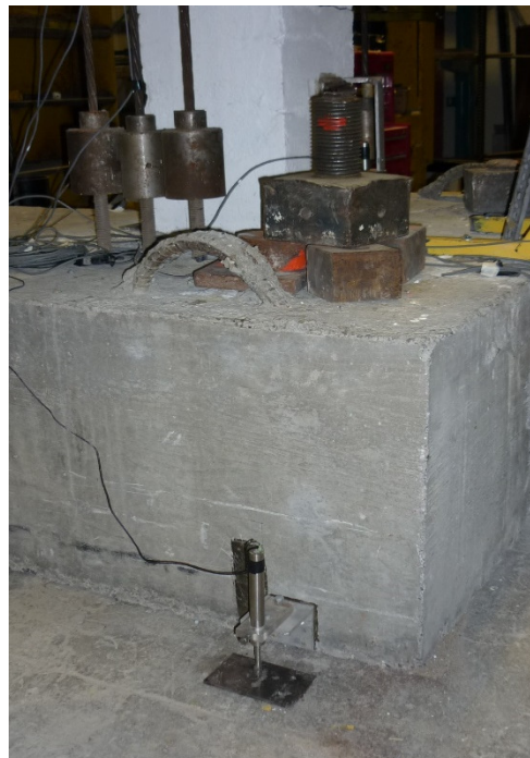
Figure 6.61: LVDT to measure uplift of foundation
