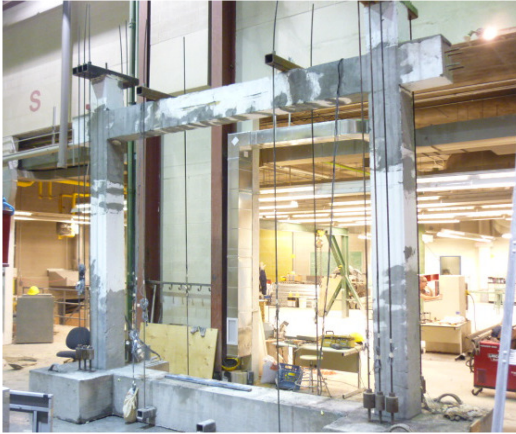
Figure 6.34: Bare control frame at end of repairing
