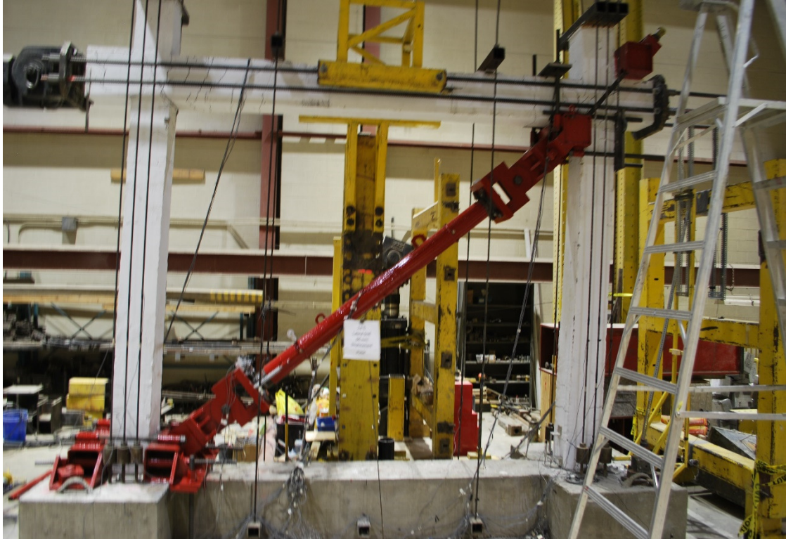
Figure 7.58: Cracking pattern at 3.0% lateral drift for Frame RRF (AISI 304 stainless steel)
