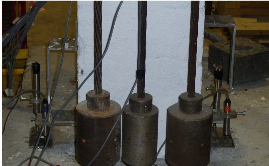
Figure 6.60: LVDT's at 25 mm and 300 mm height from foundation level to measure vertical displacements near the base
