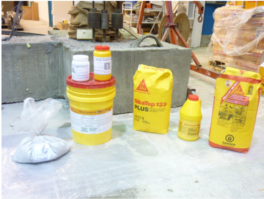
Figure 6.29: SIKA products used in the repairing process
