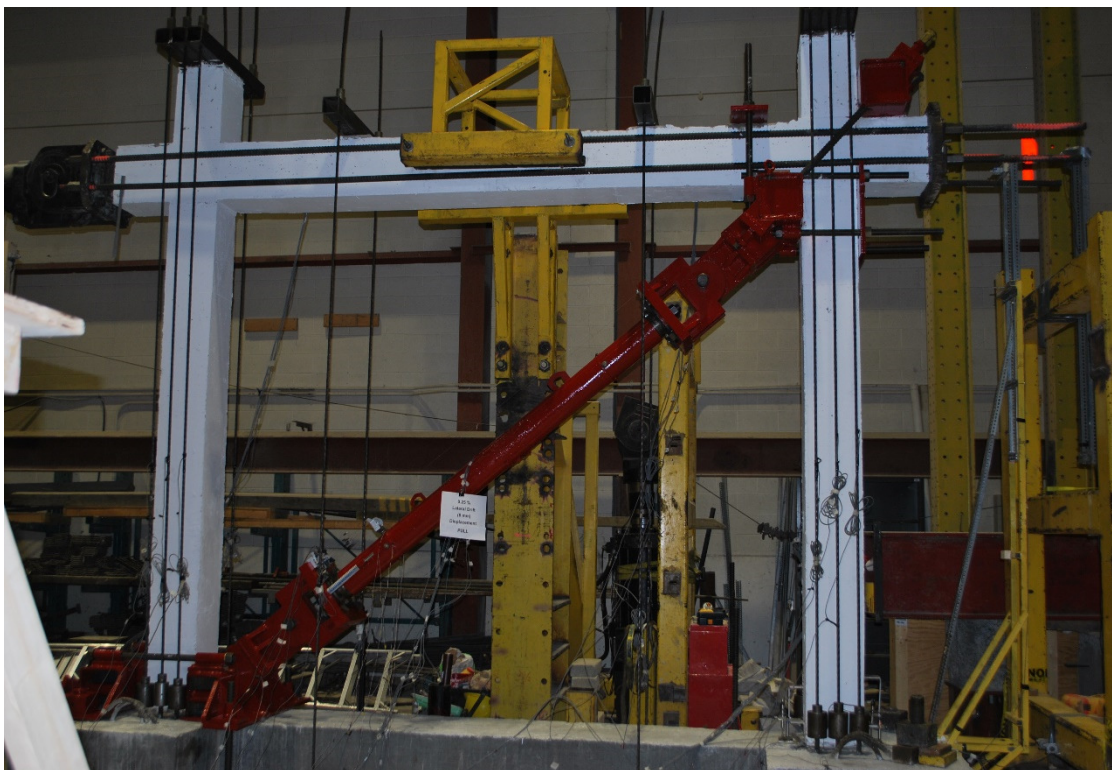
Figure 7.66: Global view at 0.25% lateral drift for Frame RF
