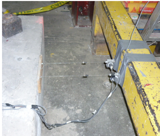
Figure 6.59: Displacement cable transducers used to measure foundation lateral displacements
