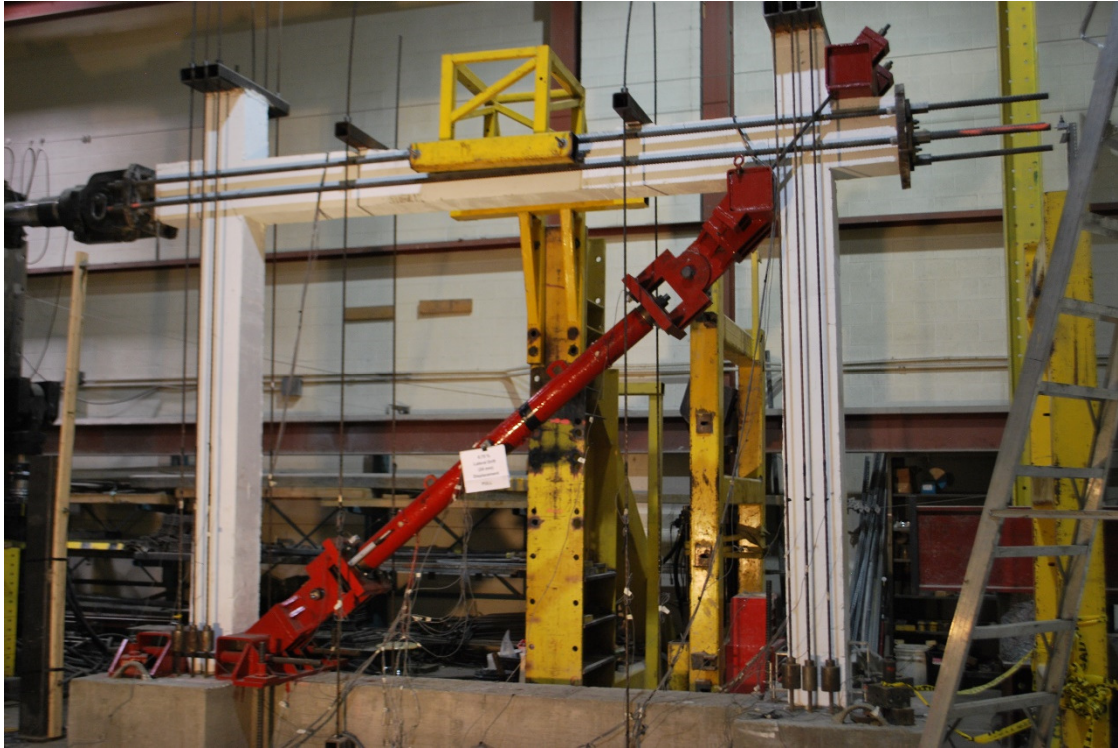
Figure 7.27: Global view at 0.625% lateral drift for Frame RRF (AISI 12L14)
