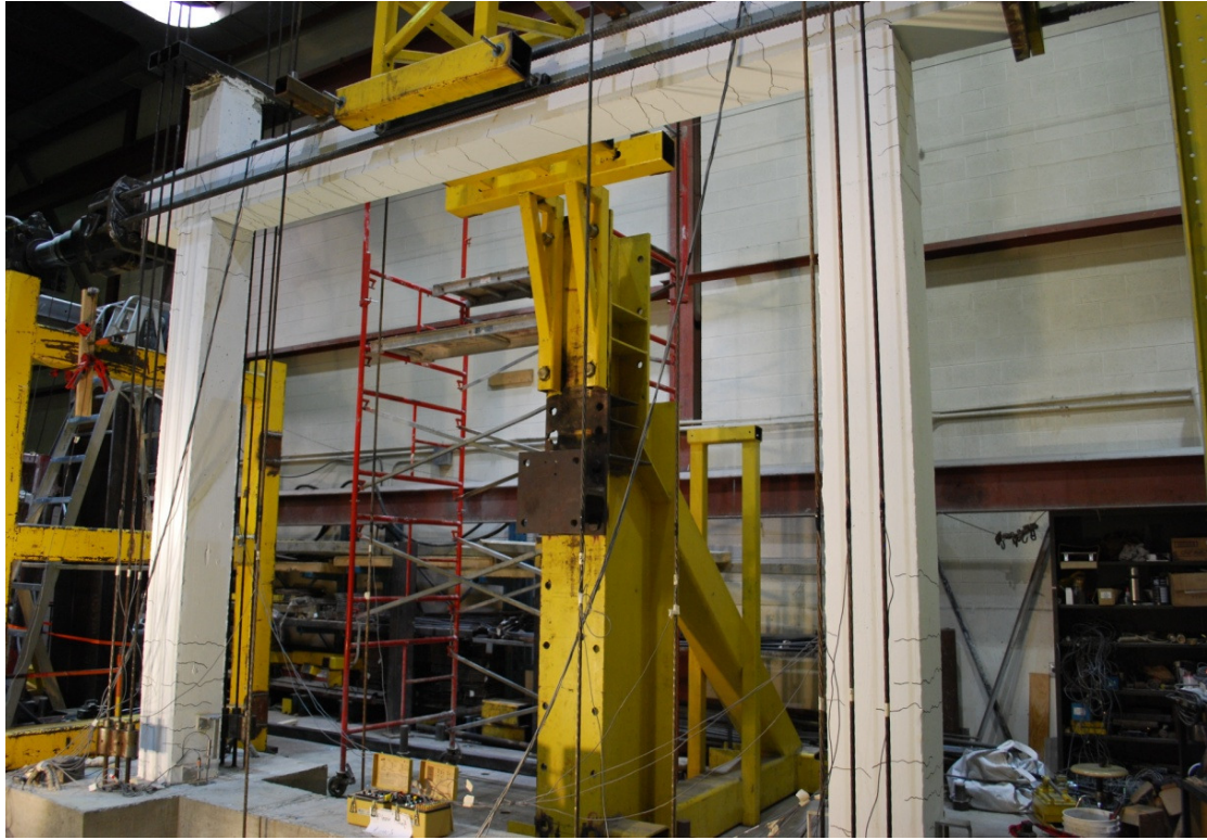
Figure 7.6: Global cracking pattern at 1.0% lateral drift for Frame BCF
