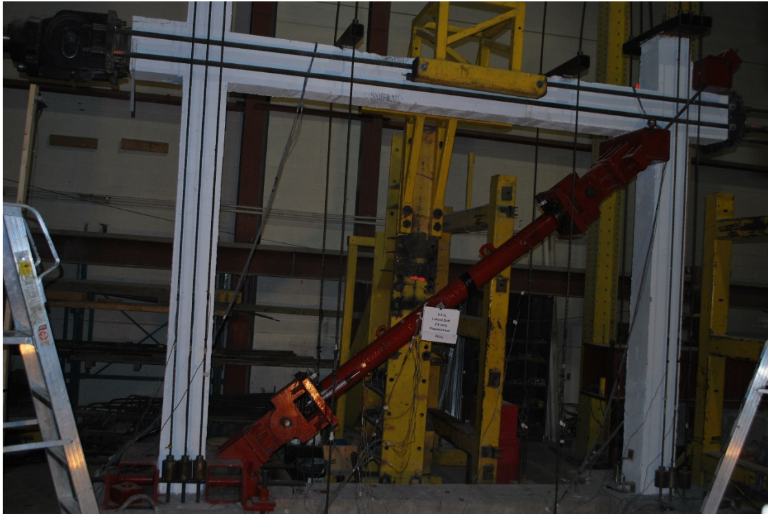
Figure 7.25: Global view at 0.5% lateral drift for Frame RRF (AISI 12L14)
