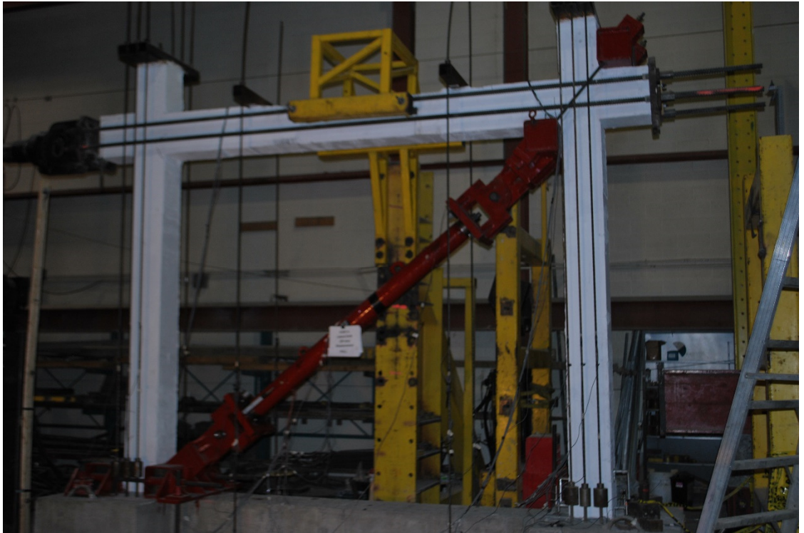
Figure 7.31: Global view at 1.0% lateral drift for Frame RRF (AISI 12L14)
