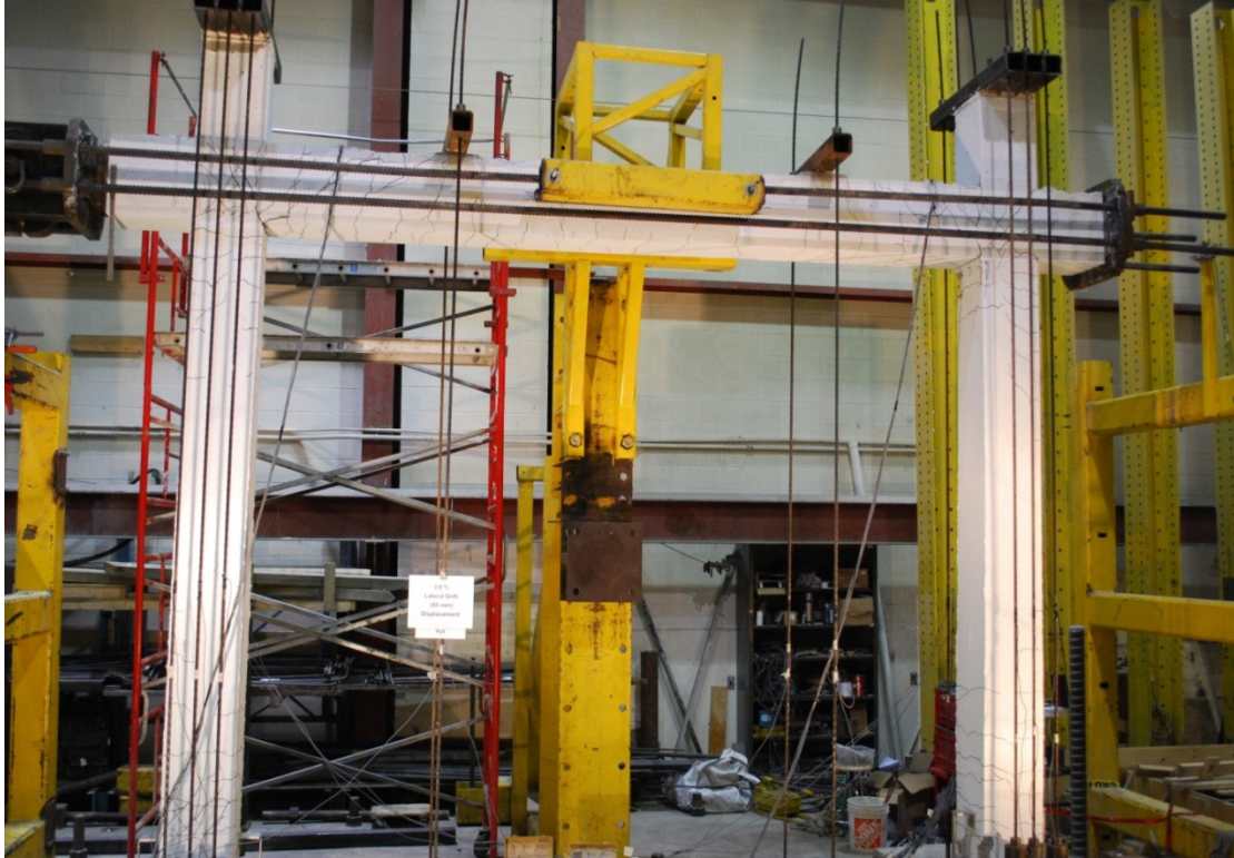
Figure 7.13: Cracking pattern at 3.0% lateral drift for Frame BCF
