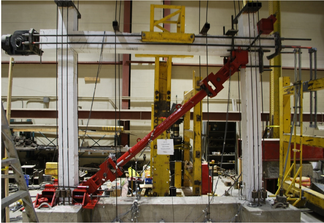
Figure 7.54: Cracking pattern at 2% lateral drift for Frame RRF (AISI 304 stainless steel)
