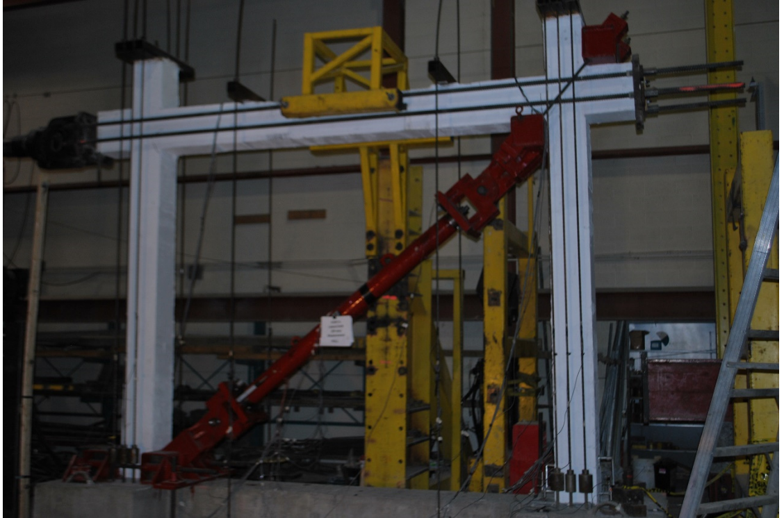
Figure 7.29: Global view at 0.75% lateral drift for Frame RRF (AISI 12L14)
