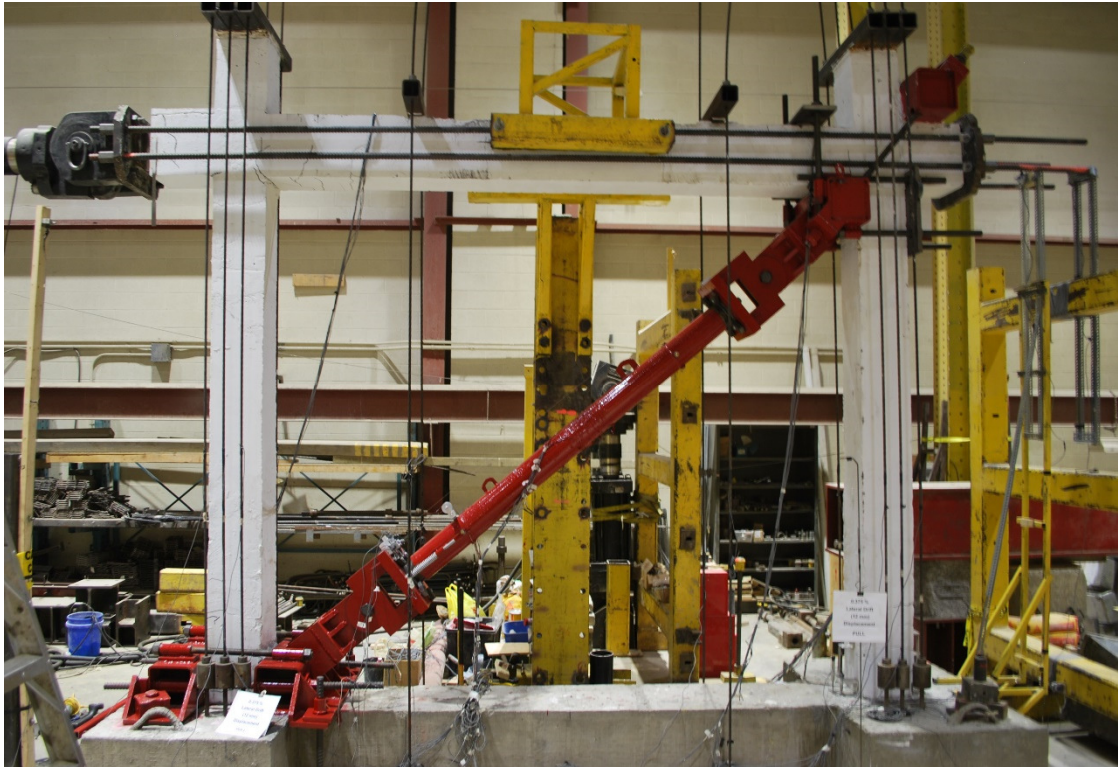
Figure 7.42: Cracking pattern at 0.375% lateral drift for Frame RRF (AISI 304 stainless steel)
