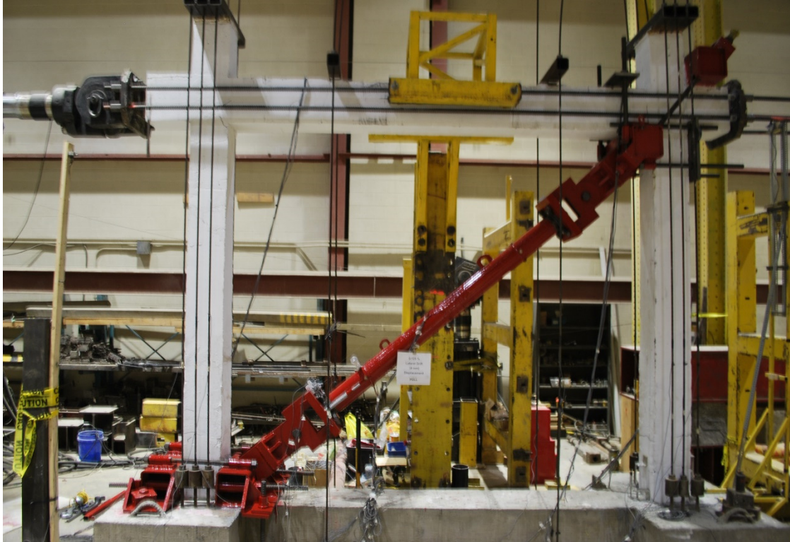
Figure 7.38: Global view at 0.125% lateral drift for Frame RRF (AISI 304 stainless steel)
