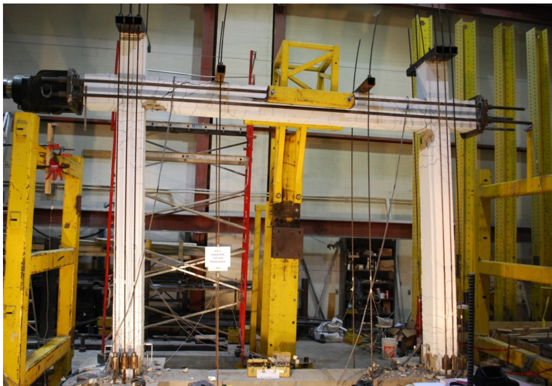
Figure 7.16: Cracking pattern and damage at 4.0% lateral drift for Frame BCF
