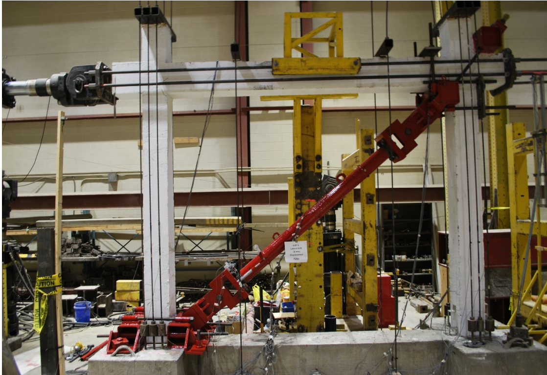
Figure 7.40: Global view at 0.25% lateral drift for Frame RRF (AISI 304 stainless steel)
