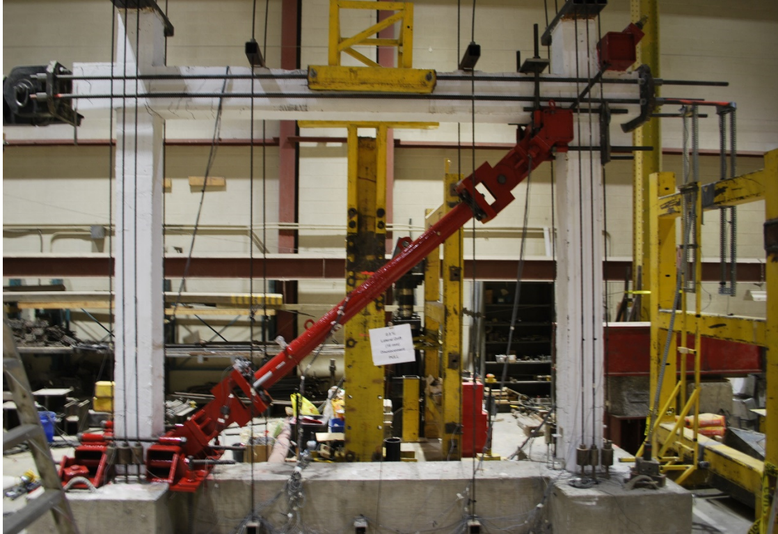
Figure 7.44: Cracking pattern at 0.5% lateral drift for Frame RRF (AISI 304 stainless steel)
