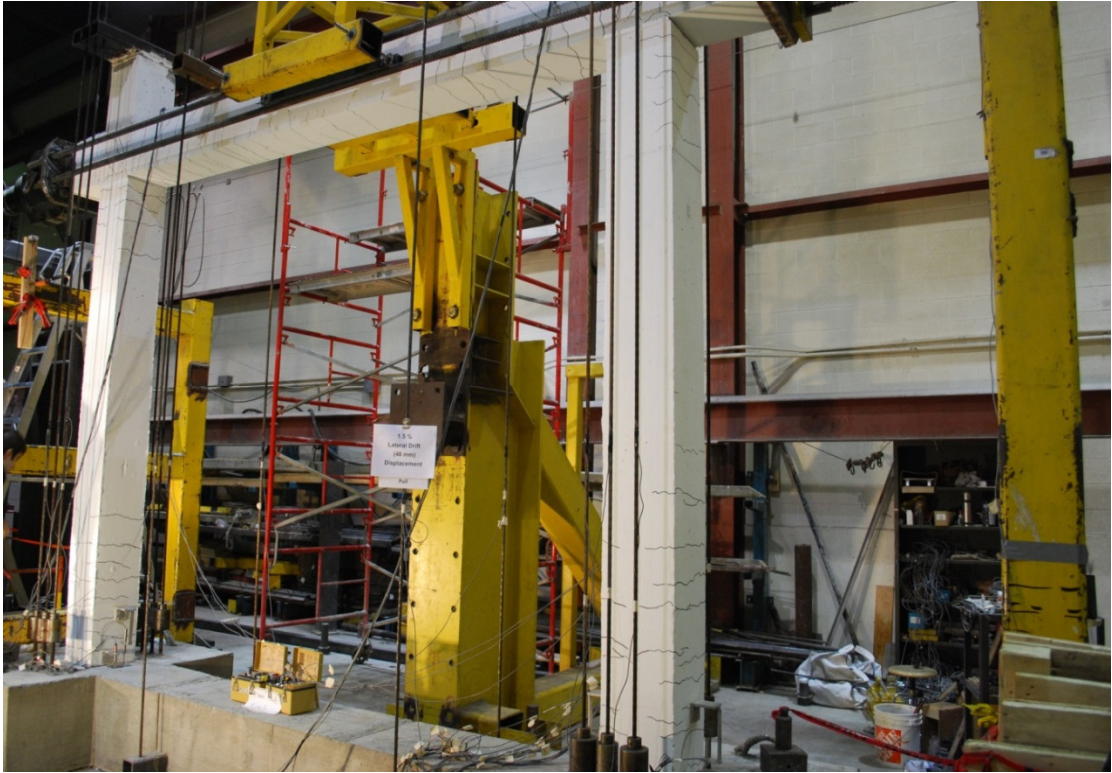
Figure 7.8: Cracking pattern at 1.5% lateral drift for Frame BCF
