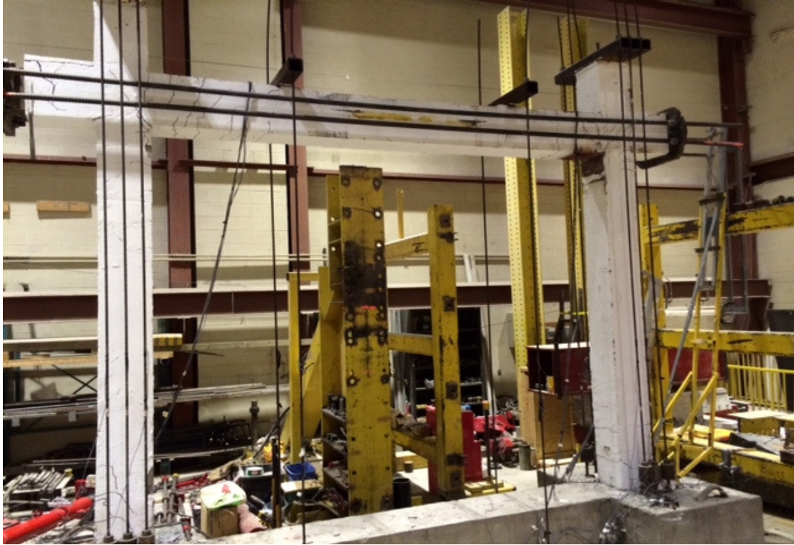
Figure 7.61: Global view of Frame RRF (AISI 304 stainless steel) after BRB removal
