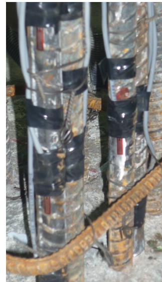
Figure 6.7: Placement of column longitudinal reinforcement and strain gauges
