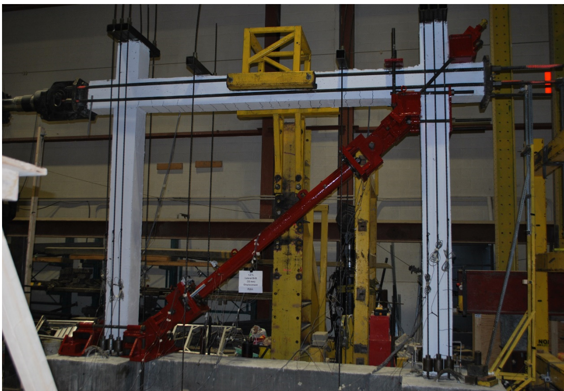
Figure 7.76: Cracking pattern at 1.0% lateral drift for Frame RF
