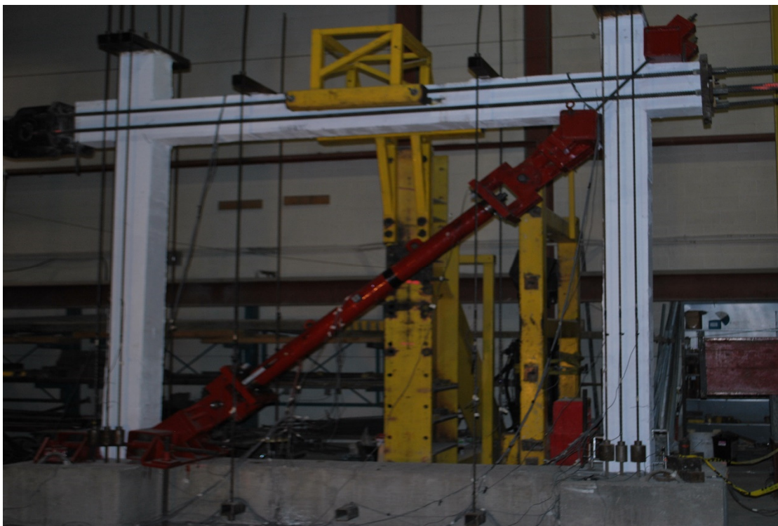
Figure 7.33: Global view at 1.5% lateral drift for Frame RRF (AISI 12L14)
