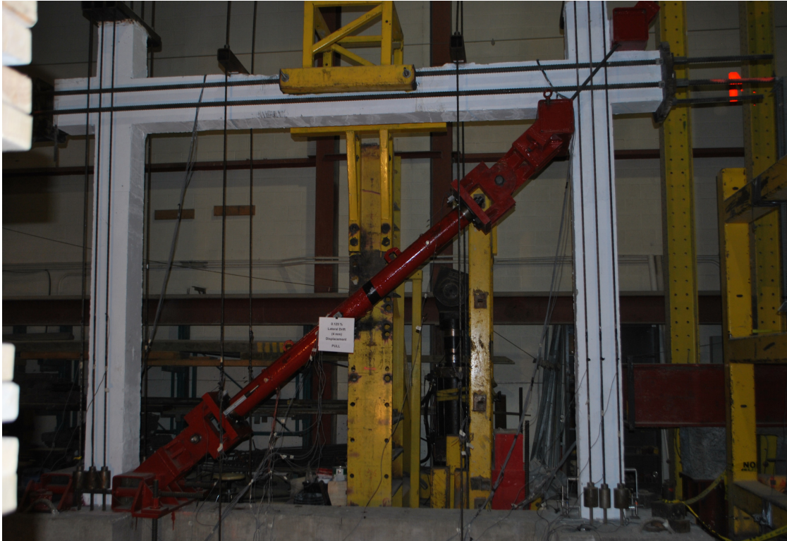
Fig. 7.19: Global view at 0.125% lateral drift for Frame RRF (AISI 12L14)
