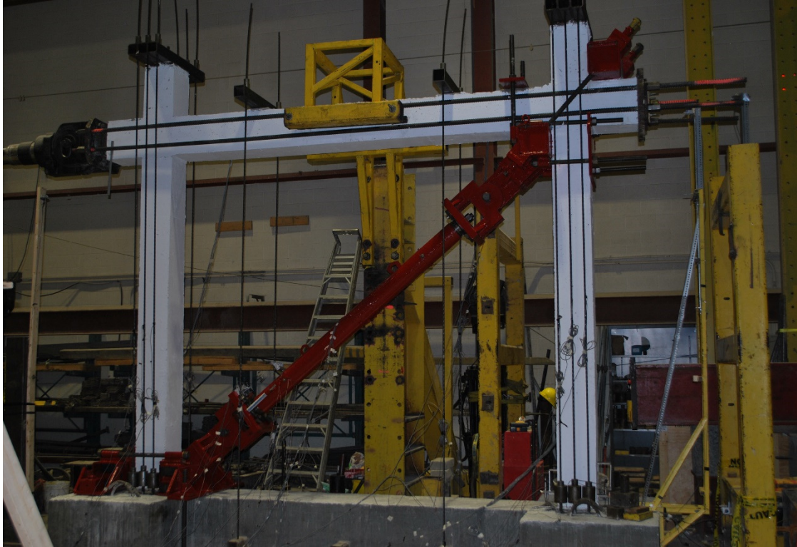
Figure 7.64: Global view at 0.125% lateral drift for Frame RF
