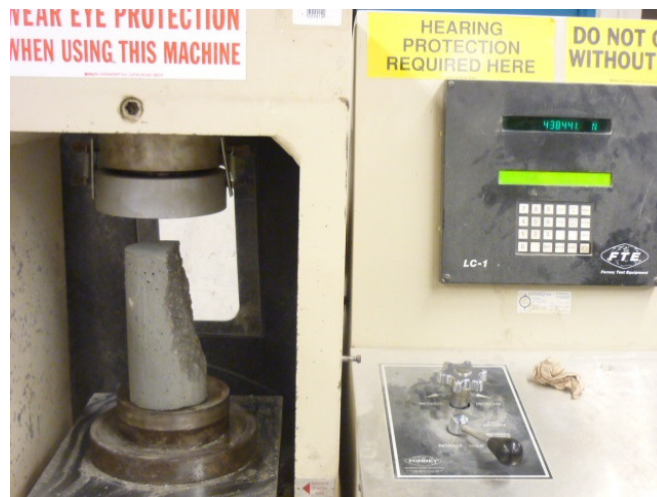
Figure 6.14: Compressive strength testing of concrete cylinders
