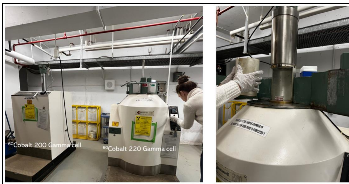
Figure 8) Irradiation setup using ^{60}\text{Co} gamma irradiators
