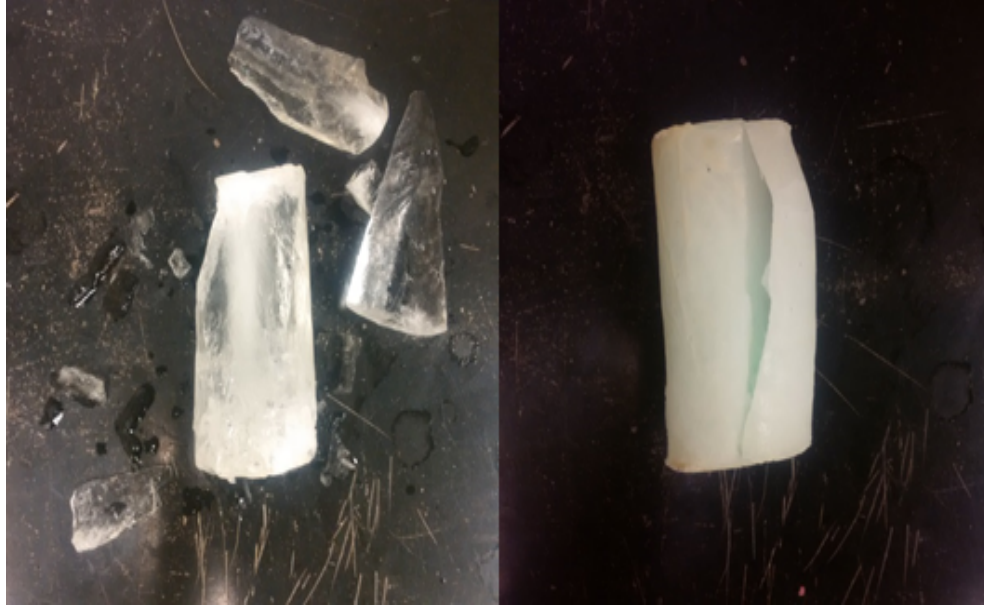
Figure 4.11: A cylinder of pure ice and a cylinder of ferrous sulphate solution samples after UCS testing.
