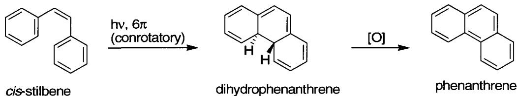
Figure 3.4 Light Induced 6\pi Conrotatory Electrocyclization of cis -Stilbene
