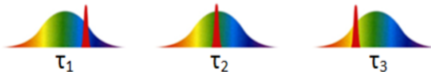
FIGURE 4.2: Schematic showing how the pump pulse (red pulse) interacts with a specific spectral component of the chirped seed (multicoloured pulse) depending on the delay between them.
