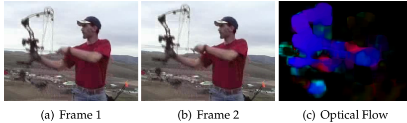
FIGURE 2.1: A simple example of the optical flow field (c), resultant from the first and second frames (a) and (b). The goal being that the background is not in the optical flow field, only the movement of subjects in the frames are considered. In this case, the only movement from frame 1 and frame 2 is a slight upward movement in the bow.
