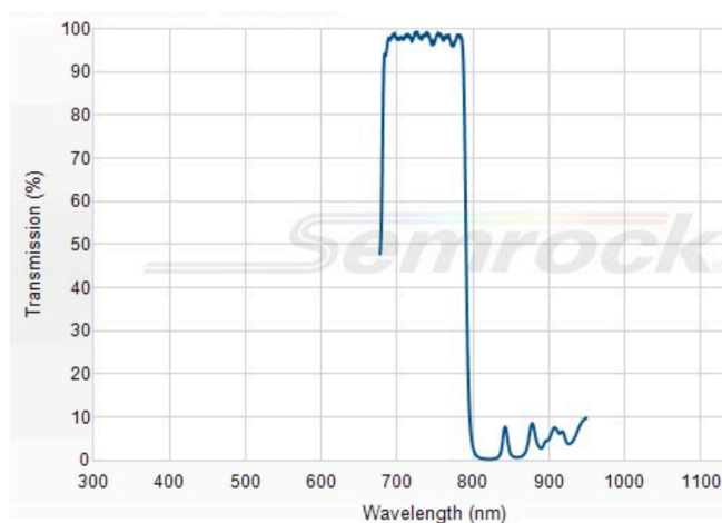
Figure 3-10 The transmission capability with an edge wavelength of 791 nm BrightLine® single-edge short-pass dichroic beamsplitter (Source: product information at Semrock®) 14 as the exciter filter or called as laser transmission filter.
