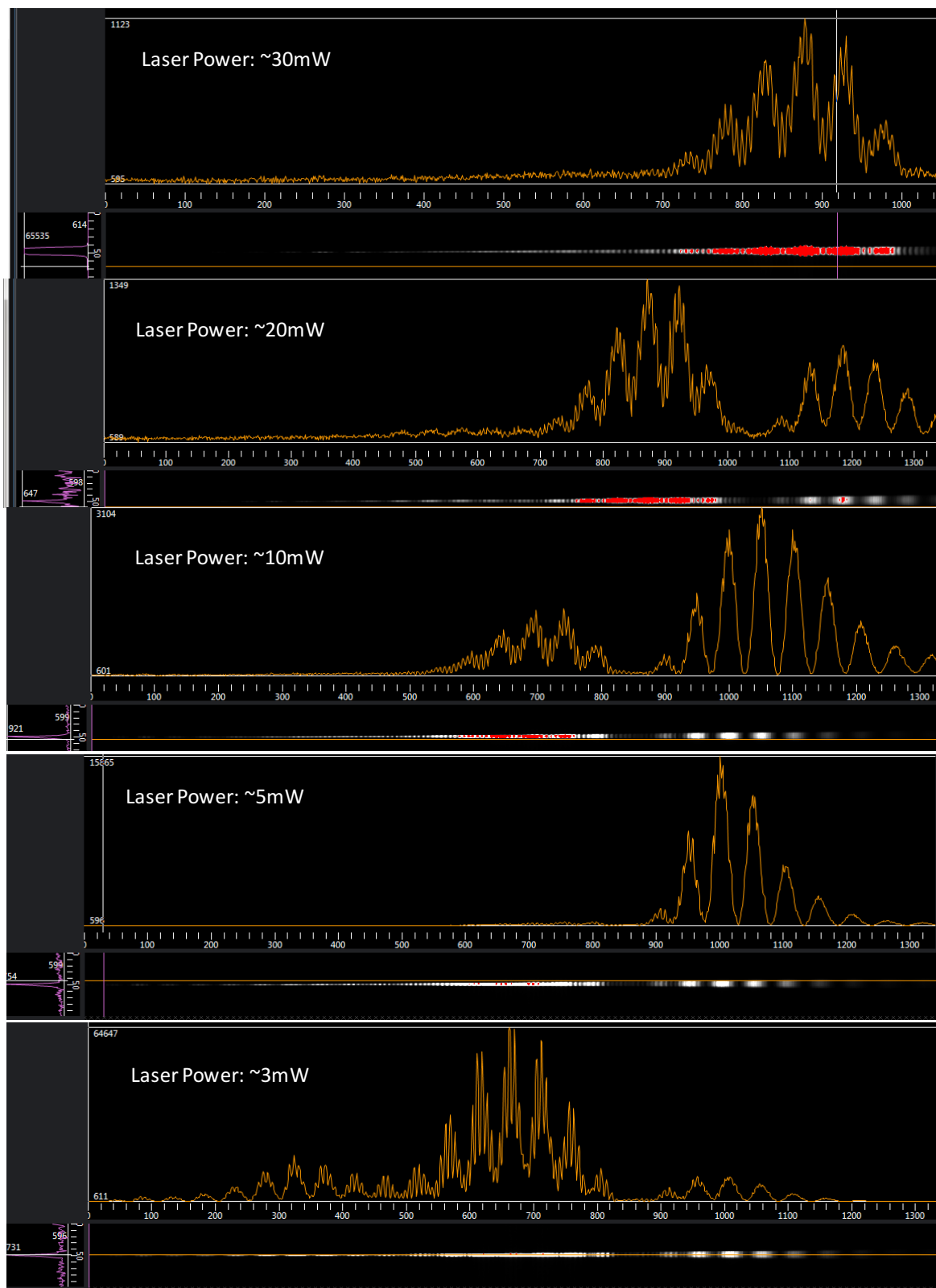
Figure 3-16 The Raman spectrums through the setup measured by the variable power of the laser with 10s of exposure time at 785 nm of both of wavelength and central wavelength.
