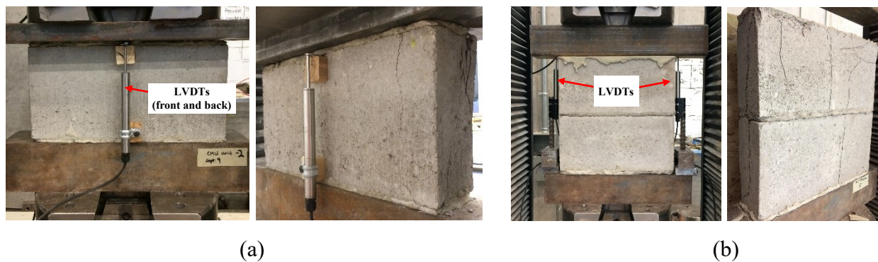
Figure 3-19. Compressive test set up, and typical failures: (a) CMU units, (b) CMU prisms Table 3-4. Compressive strength and ultimate strain of CMU blocks and prisms
