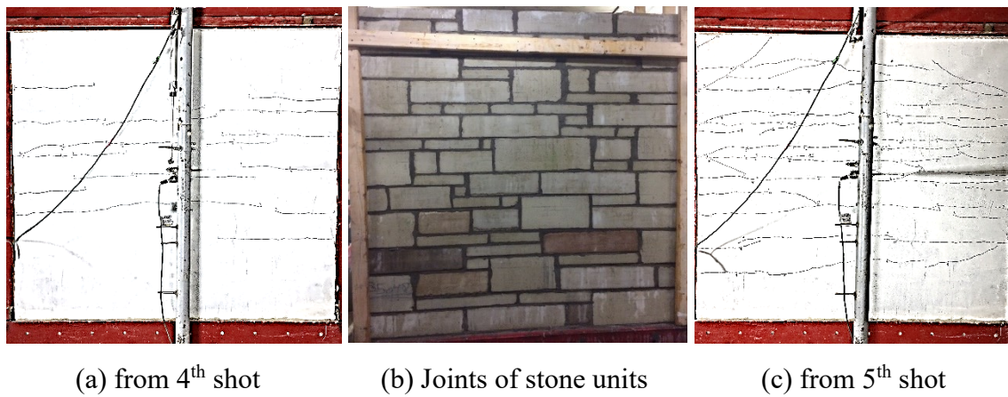
Figure 4-9. Comparison between the patterns of flexural cracks and joints of stone units
