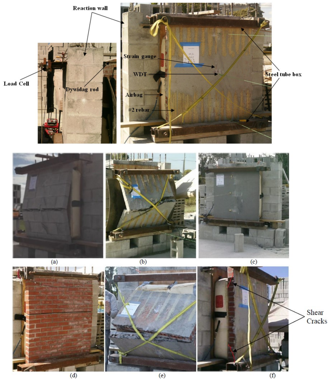
Figure 2- Failure mode of wall specimens: CMU-Control (a); CMU-1ply (b); CMU-4ply (c); CL-Control (d); CL-1ply (e); and CL-4ply (f)
