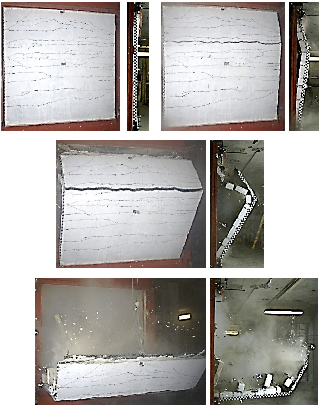
Figure 4-10. Video stills of failure mechanisms of R-S-L at the 6 th shot
