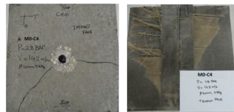
(b) Front and rear side of CFRP strengthened RC slab (129 m/s)
