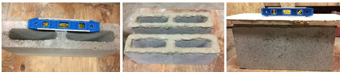
Figure 3-18. Hard capping of the specimens using high strength mortar
