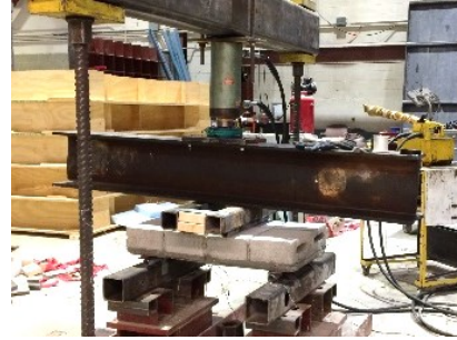
Figure 3-33. The third-point loading test setup for small beams
