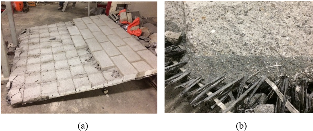
Figure 5-6. After taking the wall down: (a) Back side of the wall, (b) Interface between a CMU block and FRCM mortar
