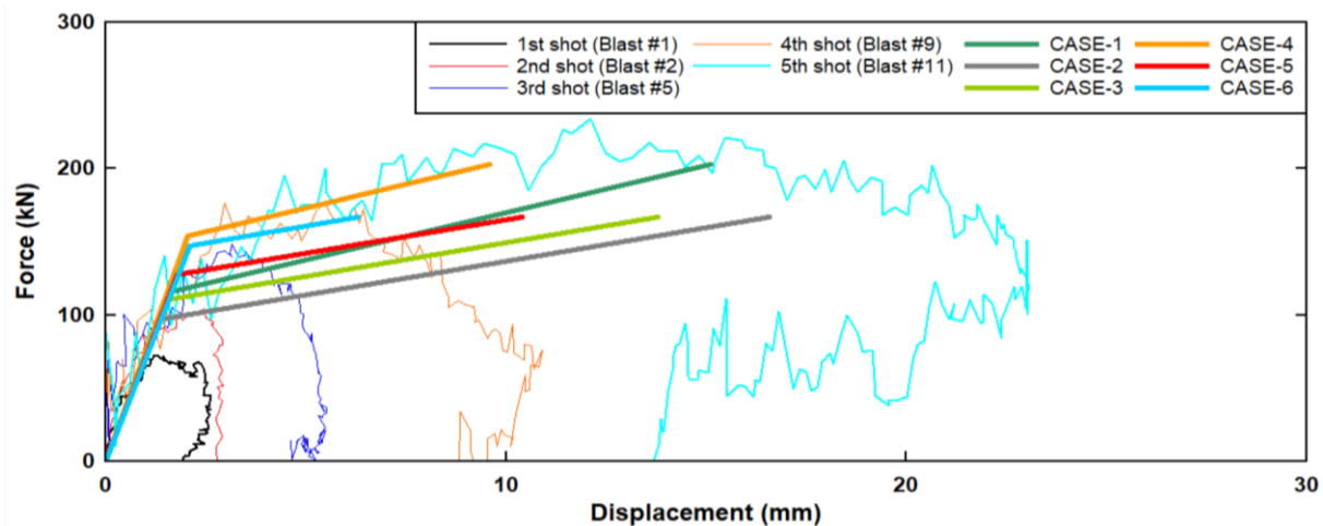
Figure 6-15. Idealized resistance curves: CASE-1 to CASE-6
