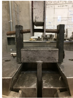
Figure 3-31. The rod bent during the 3-layer FRCM coupon test
