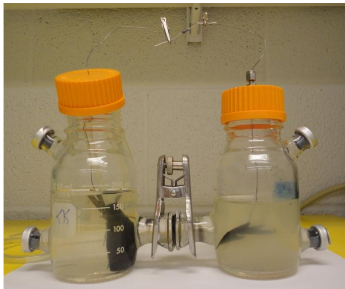
Figure 3.3. H-type MFC system. Pyrex solution bottles were used as the anode and cathode chambers.
