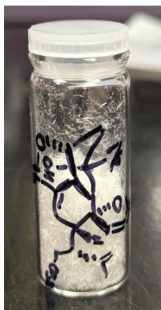
Figure 5.13. Pictures of the large-scale crystal crop from the recrystallisation of 3.53 .
