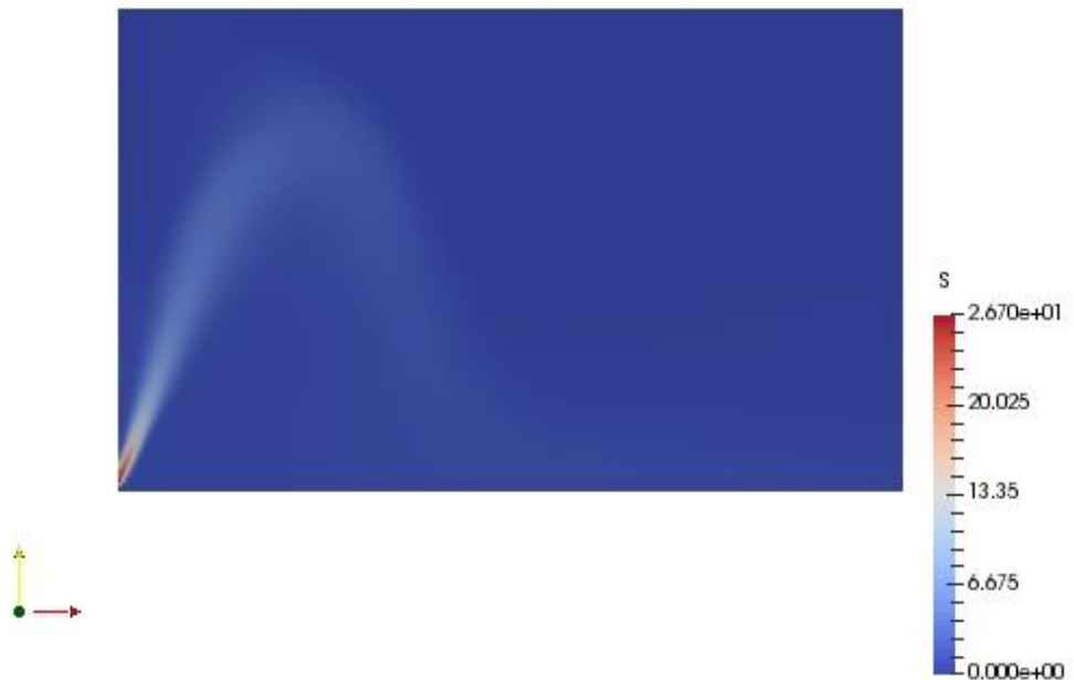
Figure 4.3: Negatively buoyant jet for 60 degrees discharge angle Froude number 50
