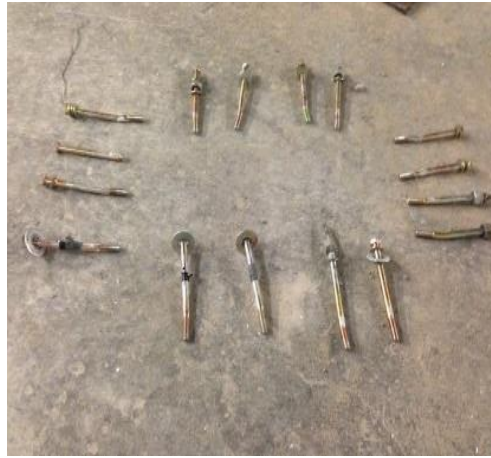
Figure 3.15: Deformed window retention anchors after test
