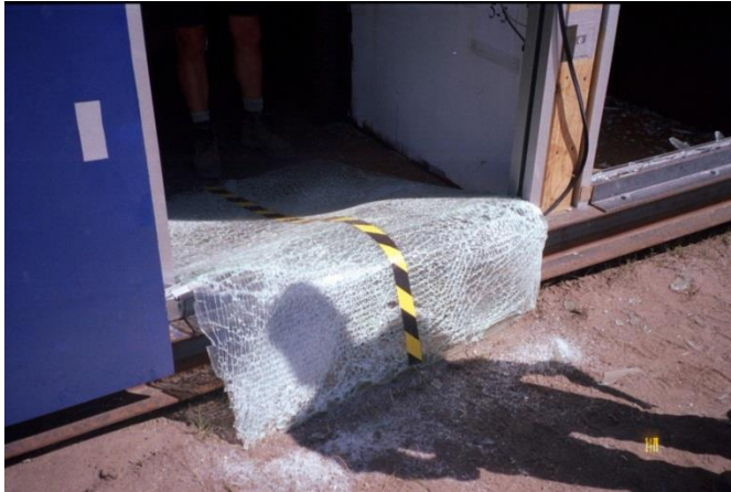
7 mill daylight film - 4psi; 30 psi-ms
