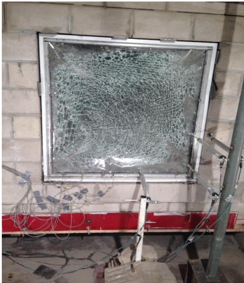
Figure B.10: Photograph of window after Test B4
