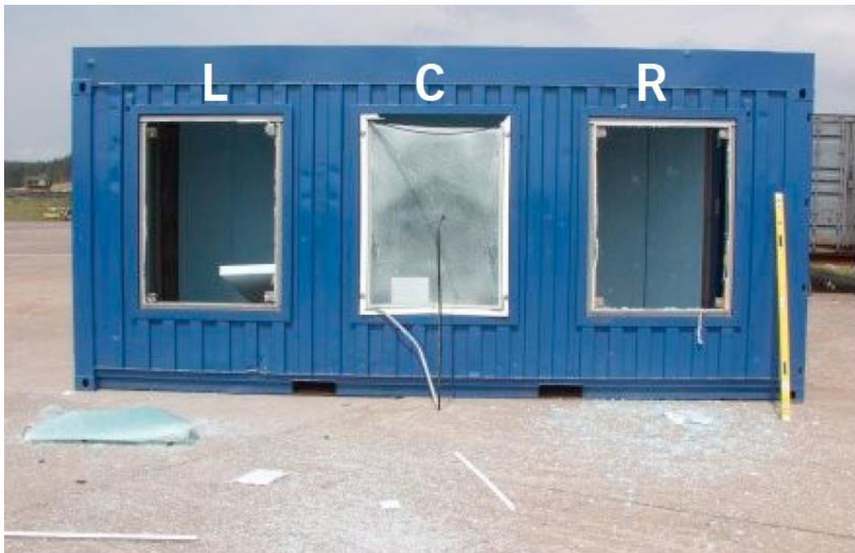
Figure 2.13: Windows L1; C2; and R3 (left, centre and right, respectively) after live testing (Panzerfilm Tests 2002)
