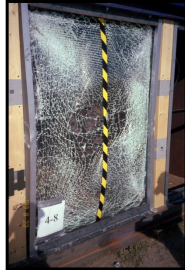
10 mill anchored film - 4 psi; 30 psi-ms
