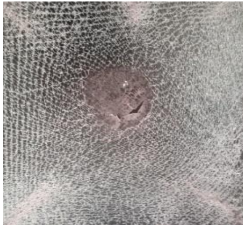
Figure 3.8: Failure of protective film
