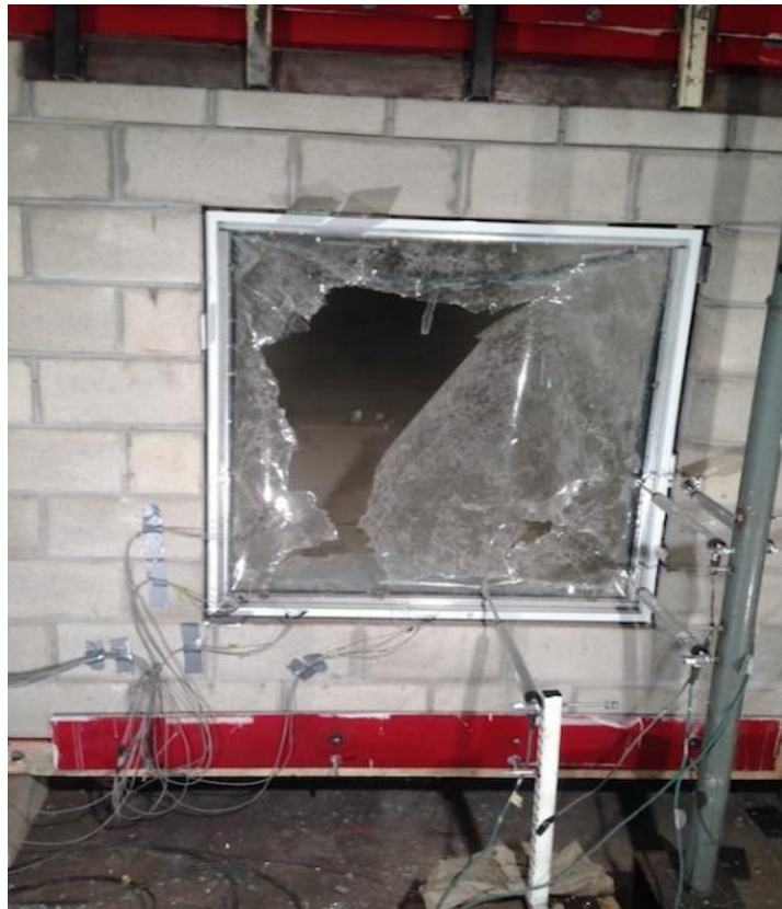
Figure B.4: Photograph of B2 after testing
