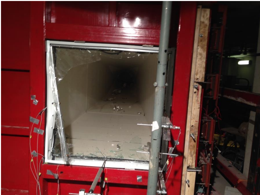
Figure A.58: Photograph of S12 after testing
