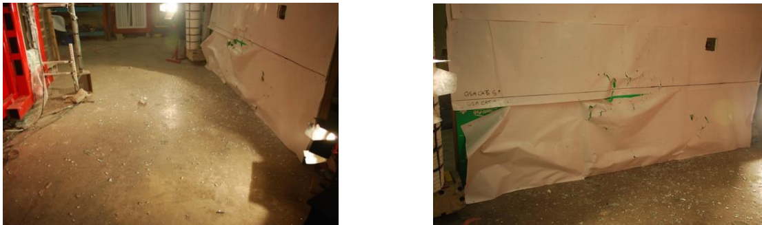
Figure A.35: Photographs of debris thrown and witness panel showing GSA demarcation line for Test S2
