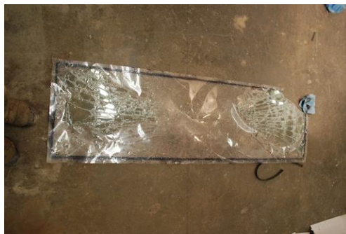
Figure A.36: Photograph of filmed window after removal, following Test S2
