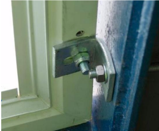
a) Gullwing profile attached to steel test cubical by means of angle brackets
