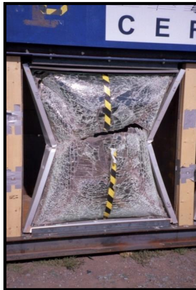
15 mil anchored film - 9 psi; 90 psi-ms
