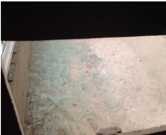
(c) Broken exterior glass inside the Shock Tube after Test C1
