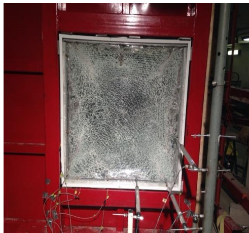
Figure 3.10: Successful performance of a glazed window
