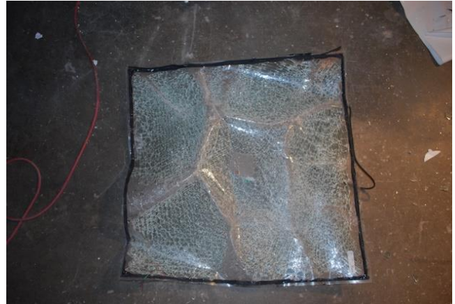
(b) Wet glazed inner pane on the floor
