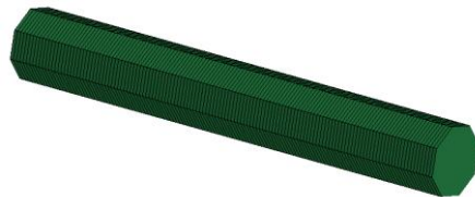
Figure C.3: Beam element mesh for anchor bolts
