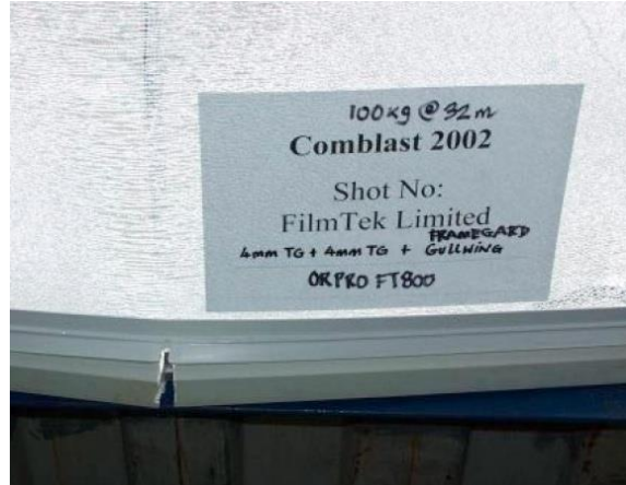
b) Rupturing of the bottom Gullwing profile
