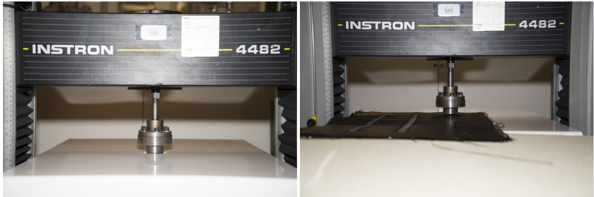
Figure 3.6: Instron testing frame configured for compaction testing. Left: sample support table fitted \sim 2.5 mm below bottom compaction platen. Right: Sample stock loaded in testing frame prior to test.
