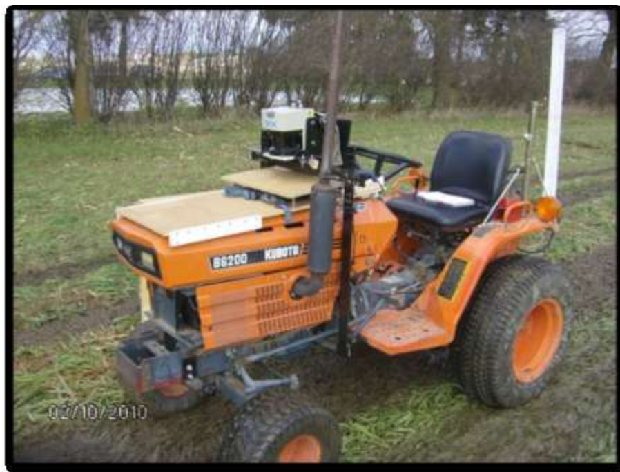
Figure 3.5: Tractor Kubota B6200 with SICK LMS 291-S14 scanner.
