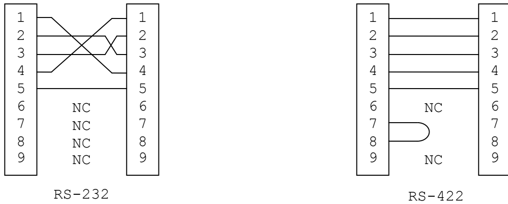
Figure 3.4: RS-232 and RS-422 serial configuration (Doerr, 2009).
