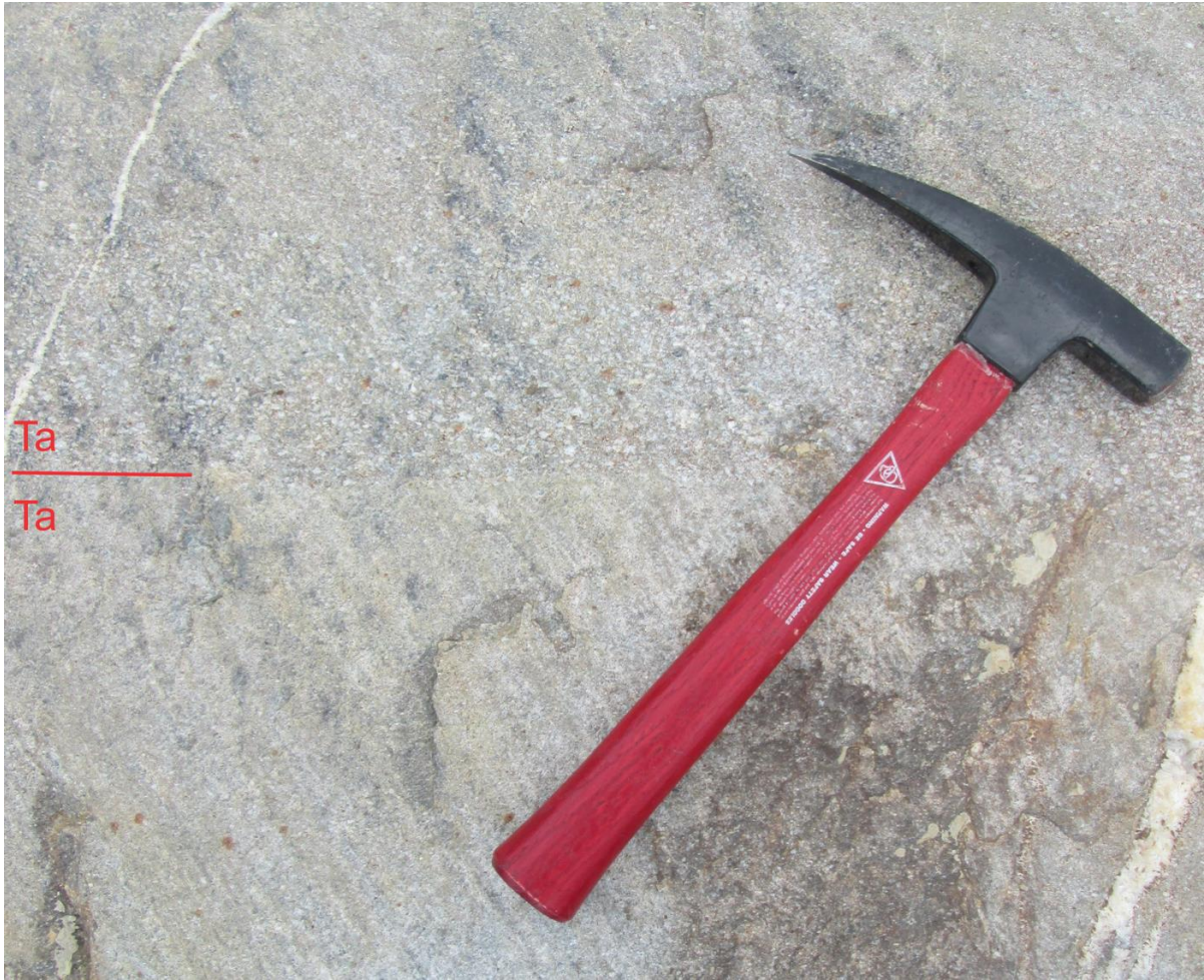
Figure 2.1: Welded contact between two Ta beds.
