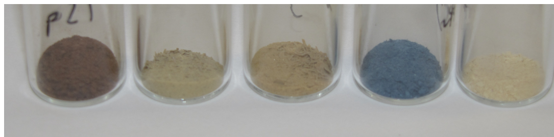
Figure 3.12 Photograph of the supports with different AgNP shapes. TiO 2 type is P90. From left to right: 1%Ag@TiO 2 (slurry method), 0.5% AgNP seeds@TiO 2 (APTES), 0.5% decahedra@TiO 2 (APTES), 0.5% plates@TiO 2 (APTES), 4% AgNO 3 @HTC
