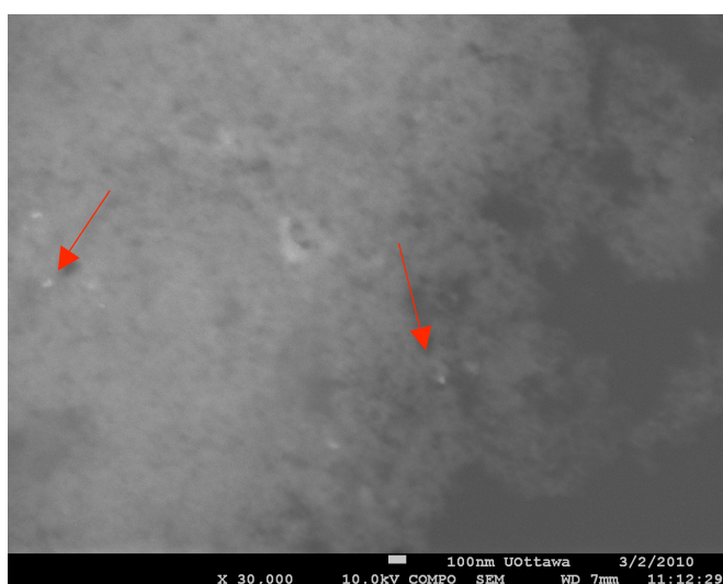
Figure 4.3 SEM image of PtNP made on \text{TiO}_2 in the slurry method. Red arrows point to the brighter spots, which are PtNP on the \text{TiO}_2 . Scale bar is 100 nm.
