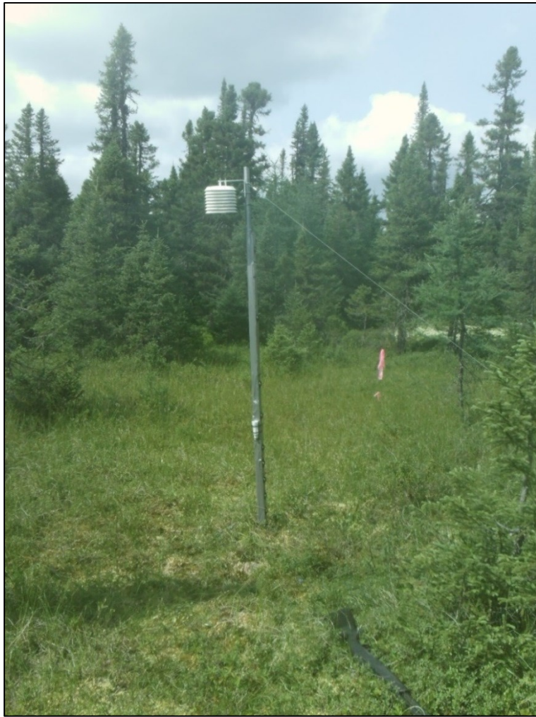
Figure 1-14: Example of a Labrador Permafrost Project monitoring station located along the Trans-Labrador Highway in eastern Labrador. Data being collected at this monitoring station include air temperature (215 cm height), ground surface temperature (1 cm depth), ground temperatures (70 cm & 120 cm depths) and snow depth.
