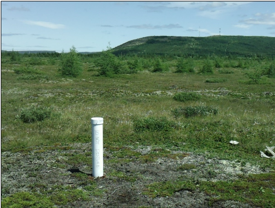
Figure 1-15: Photograph of covered borehole established at Cartwright, NL using water-jet drilling during the summer field season of 2014.
