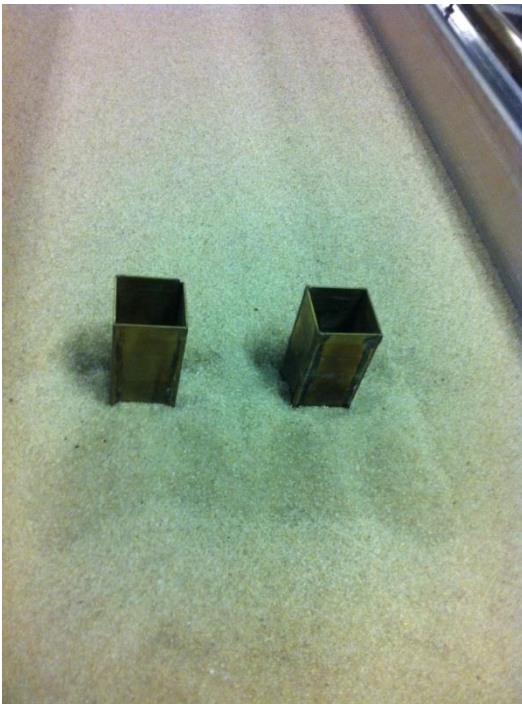
Figure 96: Small Flume - Two Square Piers
