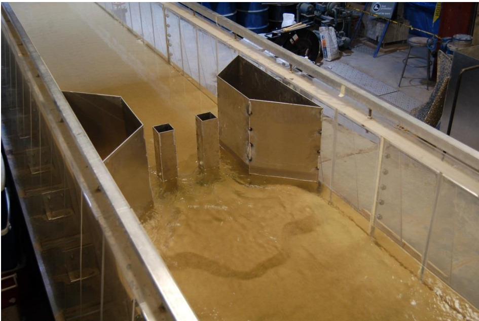
Figure 92: Photo of the Scour Pattern for the case of both the constriction and pier in the large flume
