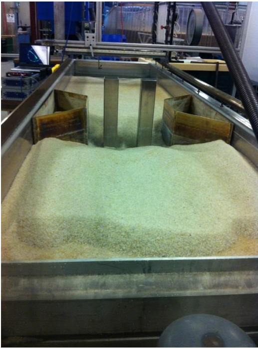
Figure 95: Small Flume- constriction and two square piers
