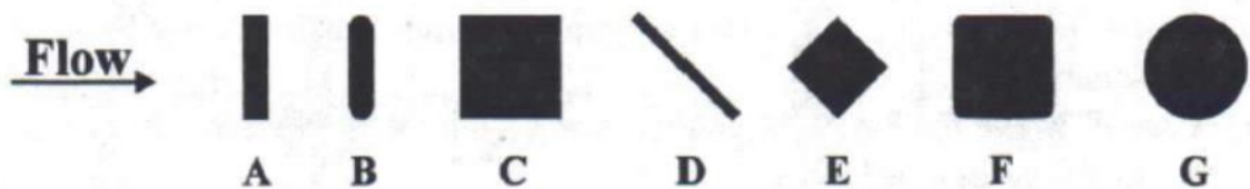
Figure 6: The shapes A to G on the scour depth relative to a circular pier (Melville, 2000)
