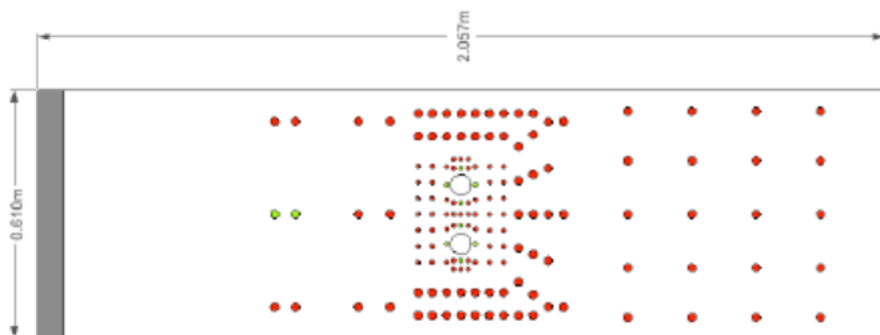
Figure 19: Planned data gathering locations for the piers only case in the small flume.
