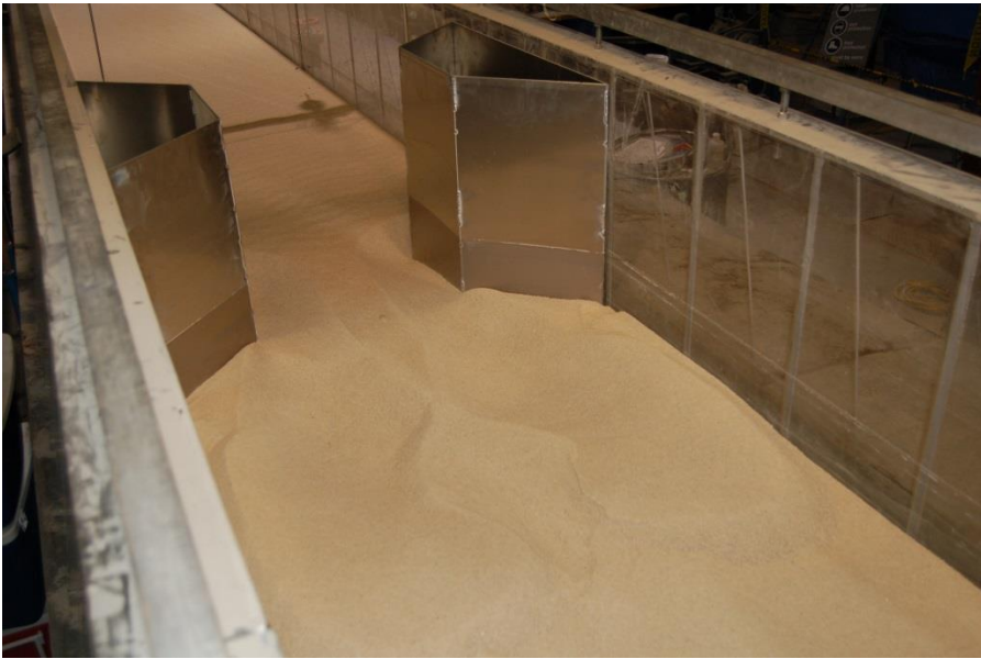
Figure 91: Photo of Scour Pattern for the case of the constriction alone in the large flume
