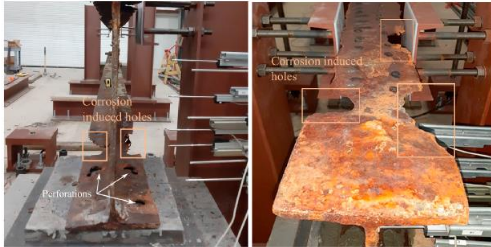
Figure 2- 2: Corroded specimen with induced holes (Tzortzinis, 2021)
