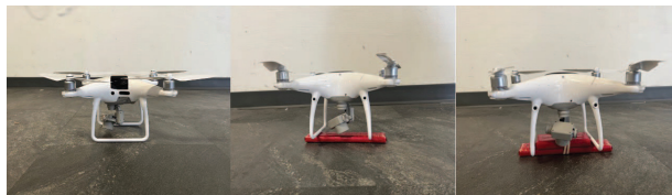
Figure 2.3: Unloaded and loaded DJI Phantom 4 (with one and two payloads) used from experimental data collection in [3] (Copyright ©2022, IEEE)
