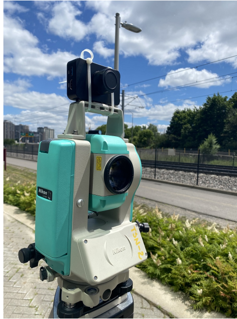
Figure 4.17: The fixed camera on the top of the TSS equipment
