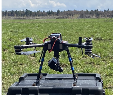
Figure 3.14: The observer drone with the mounted onboard camera
