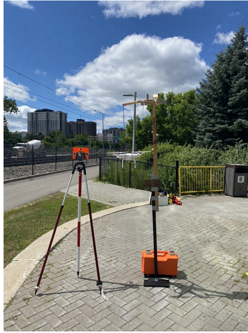
Figure 4.18: The position of the UAV close to the prism of the TSS equipment
