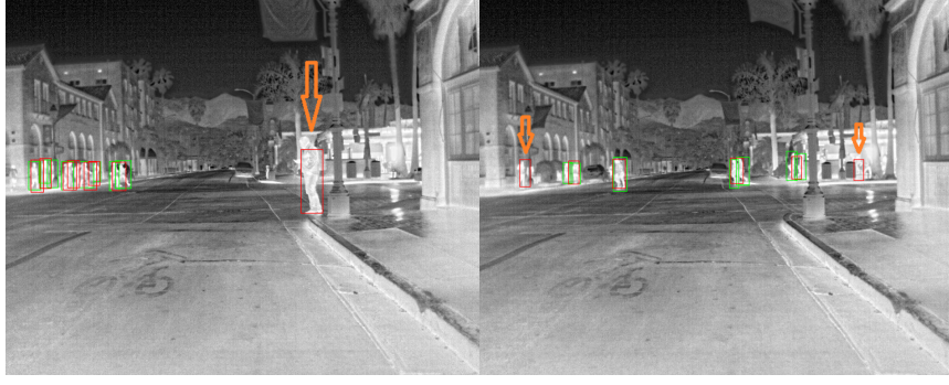
FIGURE 3.4: Samples showing missing annotations from the FLIR ADAS Dataset. Green rectangles represent ground truth boxes, red rectangles represent detected boxes, orange arrows point to instances where a pedestrian is detected by a model but no ground truth annotation exists.
