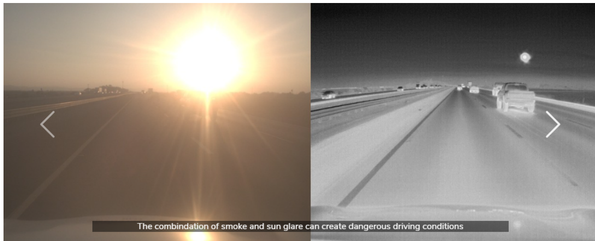
FIGURE 1.2: Images of a scene taken using an RGB camera (left) and thermal camera (right). The thermal image is not at all affected with the glare from the sun, while the RGB camera is significantly affected and the truck can barely be seen.
