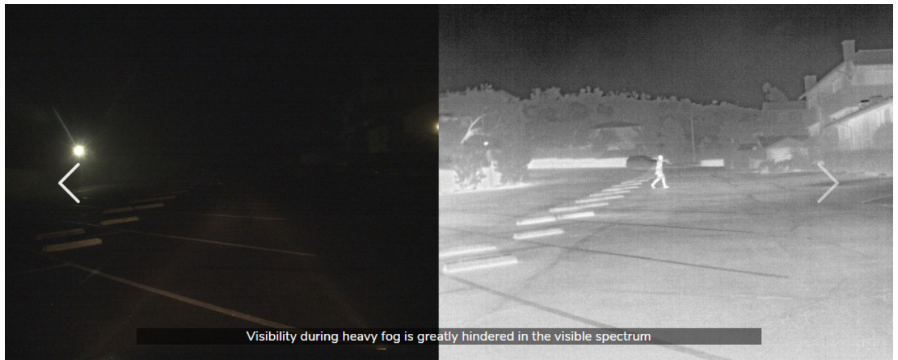
FIGURE 1.1: Images of a scene taken using an RGB camera (left) and thermal camera (right). The pedestrian and vehicle are almost entirely non visible in the RGB image, while they are clearly visible in the thermal image.
